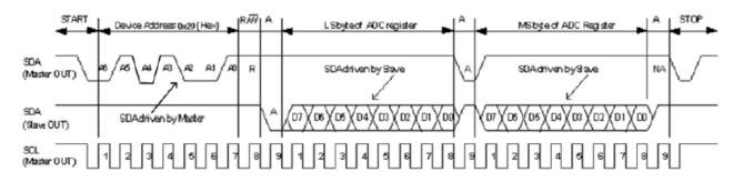
Figure 16. I<sup>2</sup>C Timing Diagram for Receive Word Format
