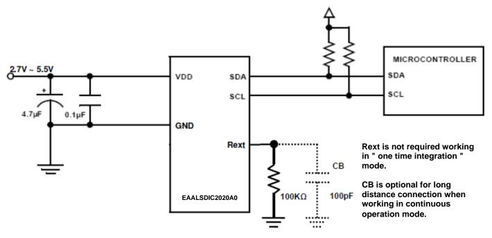
Figure 17. Application Circuit
