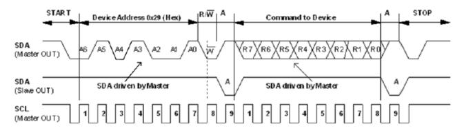
Figure 14. I<sup>2</sup>C Timing Diagram for Send Byte Format
