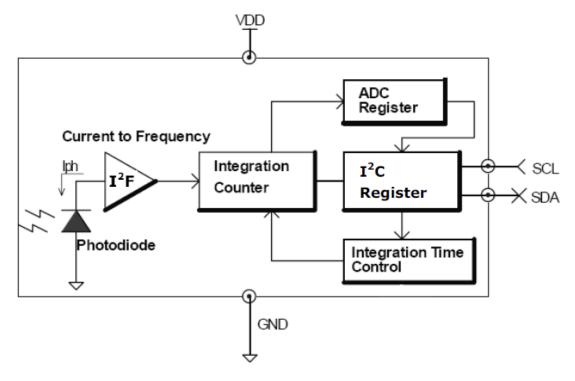
Figure 1. EAALSDIC2020A0 Functional Block Diagram
