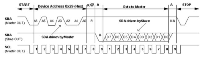
Figure 15. I<sup>2</sup>C Timing Diagram for Receive Byte Format
