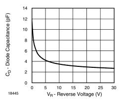
Fig. 4 - Typical Capacitance vs. Reverse Voltage
