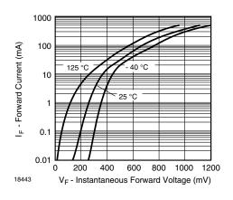
Fig. 2 - Typical Forward Characteristics
