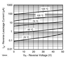
Fig. 3 - Typical Reverse Characteristics
