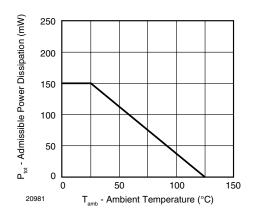
Fig. 1 - Admissible Power Dissipation vs. Ambient Temperature
