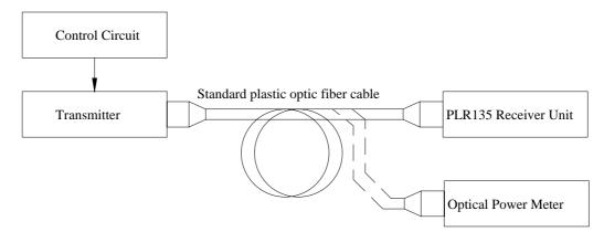
\*Fig.2 Measuring Method of Dissipation Current
