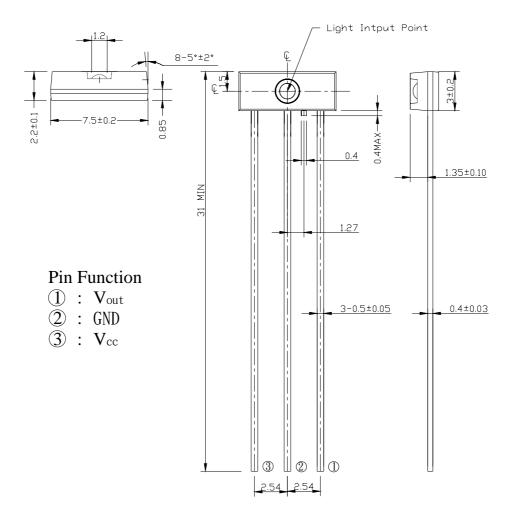
Notes: 1.All dimensions are in mm. 2.General Tolerance: Pin length tolerance is  $\pm 0.25$  mm others are  $\pm 0.10$  mm
