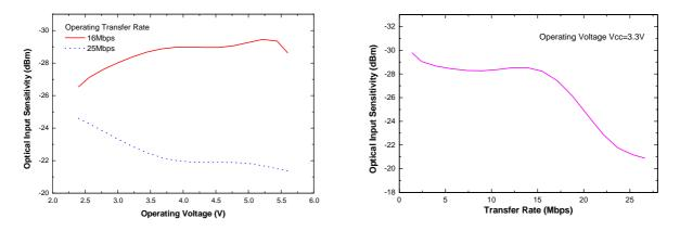
**Note:** Before using the PLR135 device, please confirm the minimum sensitivity at different operating voltage and transmission rate.
