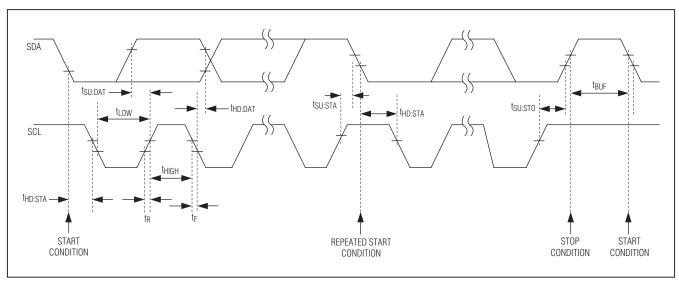
Figure 1. SMBus Timing Diagram
