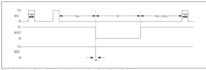
Figure 5. Watchdog Startup Sequence with Watchdog Reset Output Enable Bit Set to '1'
