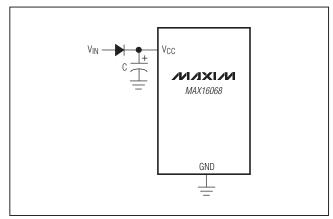
Figure 12. Power Circuit for Shutdown During Fault Conditions
