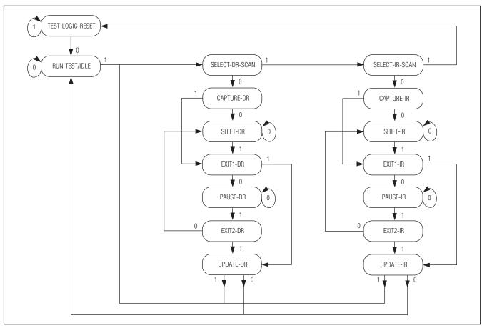
Figure 11. Tap Controller State Diagram
