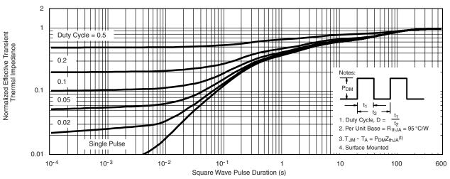
Normalized Thermal Transient Impedance, Junction-to-Ambient
