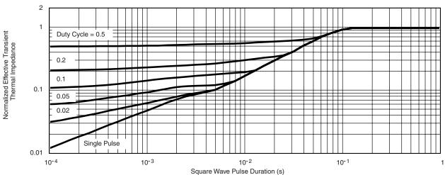
Normalized Thermal Transient Impedance, Junction-to-Foot
