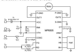
Figure 4: Detailed Application Schematic
