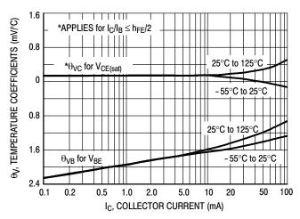
**Figure 10. Temperature Coefficients**
