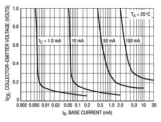
Figure 7. Collector Saturation Region
