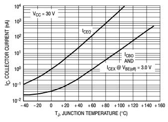
Figure 19. Typical Collector Leakage Current
