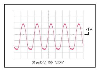
Divide-by-2048 Output (Input: 10 GHz; Output: 4.9 MHz)
