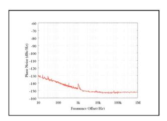
Divide-by-(8/3) Output (Input: 10 GHz; Output: 3.75 GHz)
