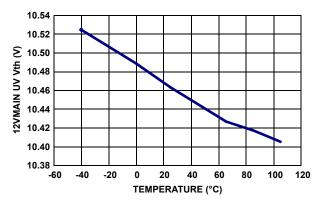
FIGURE 29. 12VMAIN POWER GOOD THRESHOLD VOLTAGE VS TEMPERATURE
