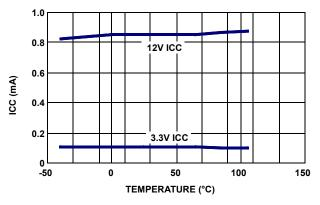
FIGURE 22. ICC CURRENT vs TEMPERATURE
