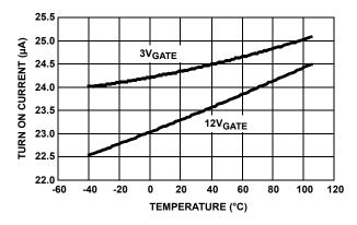
FIGURE 31. ISL6113 GATE TURN-ON CURRENT (ABS) vs TEMPERATURE
