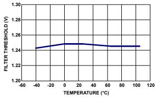
FIGURE 35. FILTER THRESHOLD VOLTAGE vs TEMPERATURE
