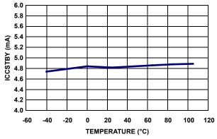
FIGURE 21. ICCSTBY CURRENT vs TEMPERATURE
