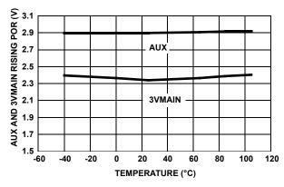
FIGURE 28. AUX AND 3VMAIN RISING POR THRESHOLD VOLTAGE vs TEMPERATURE
