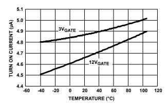
FIGURE 32. ISL6114 GATE TURN-ON CURRENT (ABS)
