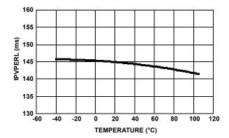
FIGURE 36.  $t_{PVPERL}$  vs TEMPERATURE
