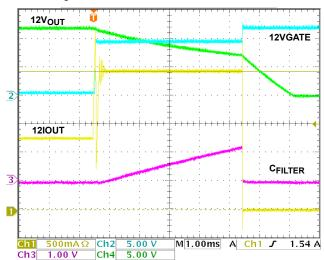
FIGURE 12. ISL6113 12VMAIN CR AND SHUTDOWN
