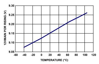
FIGURE 27. 12VMAIN RISING POR THRESHOLD VOLTAGE VS TEMPERATURE
