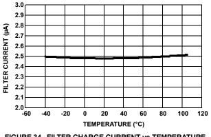
FIGURE 34. FILTER CHARGE CURRENT vs TEMPERATURE
