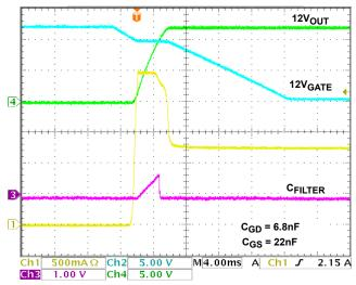
FIGURE 3. ISL6113 12VMAIN START-UP  $R_{LOAD}$  = 10 $\Omega$ ,  $C_{LOAD}$  = 470 $\mu F$
