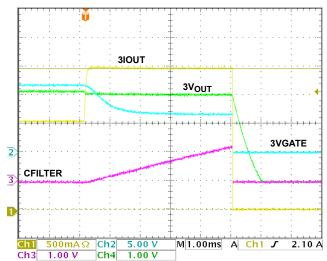
FIGURE 13. ISL6113 3VMAIN CR AND SHUTDOWN
