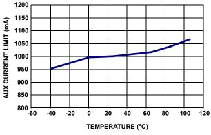
FIGURE 25. AUX CURRENT LIMIT vs TEMPERATURE
