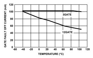
FIGURE 33. GATE FAULT OFF CURRENT (ABS) vs TEMPERATURE
