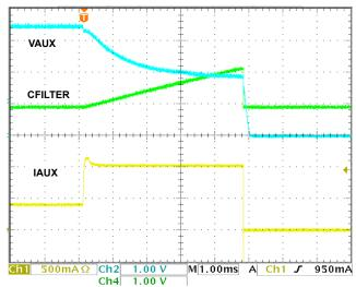
FIGURE 16. VAUX OC REGULATION AND SHUTDOWN
