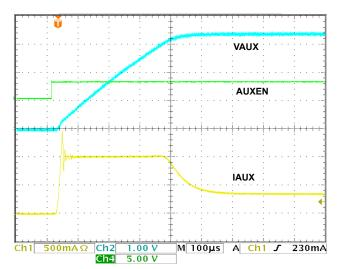
FIGURE 2. VAUX TURN-ON R<sub>LOAD</sub> =  $10\Omega$ , C<sub>LOAD</sub> =  $100\mu$ F
