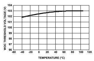
FIGURE 24. FAST TRIP THRESHOLD VOLTAGE VS TEMPERATURE
