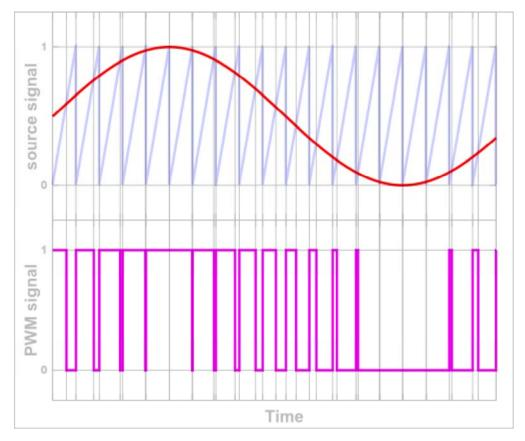
This PWM signal is clocked at 250kHz, which is much higher than the audio frequencies being encoded (< 20kHz). Because speakers are mechanical devices that can only respond to audio frequencies, the PWM signal is effectively filtered back into the original audio frequencies by the speaker coil itself. All you hear is the music!
