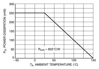
Figure 1. Derating Curve
