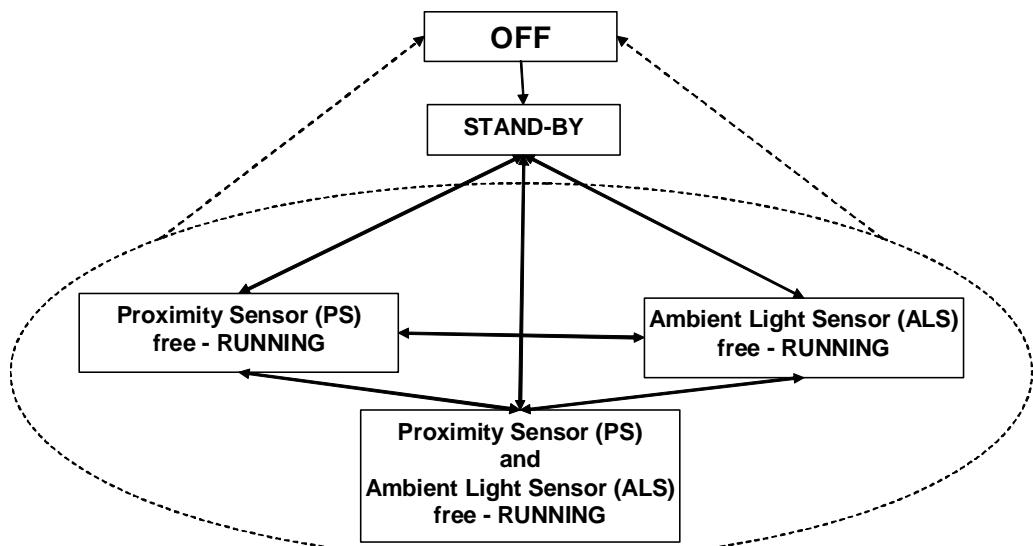
If  $V_{DD}$  exceeds the threshold voltage, the sensor will switch from OFF mode to STAND-BY mode. As shown in the transition-diagram above it is possible to switch between all modes without any restriction.
