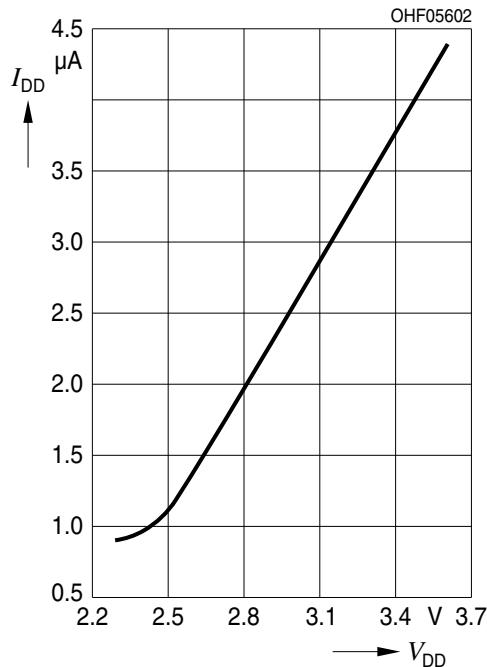
**Current consumption  $I_{DD}$  in PS mode**
