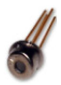
These products are high-performance 850nm VCSELs (Vertical Cavity Surface-Emitting Lasers) designed for high-speed data communications and packaged with a custom designed power monitor diode. The power monitor diode can be used with appropriate feedback control circuitry to set a maximum power level for the VCSEL. These combined features simplify design for high data rate communication and eye safety.
