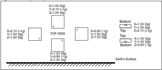
Figure 4 refers to the LIS332AR powered at 3 V.
