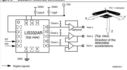
Power supply decoupling capacitors (100 nF ceramic or polyester + 10  $\mu$ F aluminum) should be placed as near as possible to the device (common design practice).
