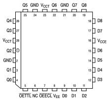
Figure 1. PLCC-28 Pinout (Top View)
