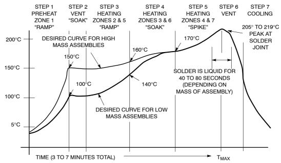
Figure 61. Typical Tin Lead (SnPb) Solder Heating Profile
