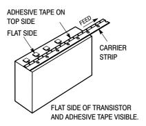
Style M fan fold box is equivalent to styles E and F of reel pack dependent on feed orientation from box.
