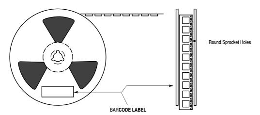
Figure 43. Round Sprocket Holes Used with 8 mm, 12 mm,16 mm and 24 mm Tape (holes on one side only)
