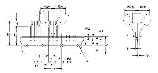
Figure 44. Device Positioning on Tape
