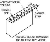
Style P fan fold box is equivalent to styles A and B of reel pack dependent on feed orientation from box.
