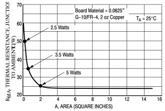
Figure 59. Thermal Resistance versus Drain Pad Area for the D<sup>2</sup>PAK Package (Typical)
