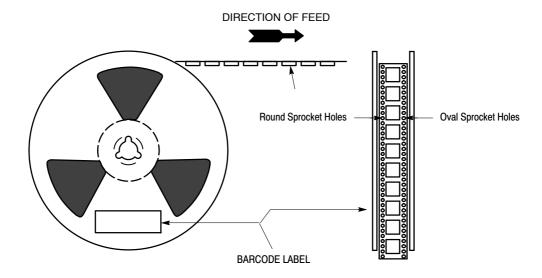
Figure 42. Round and Oval Sprocket Holes Used with 32 mm, 42 mm, 44 mm and 52 mm Tape (holes on both sides)
