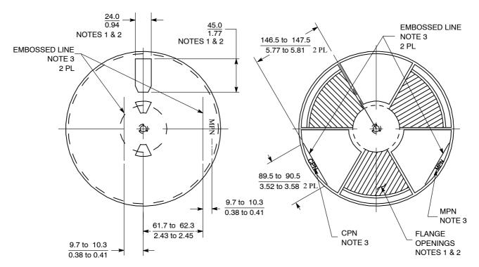
Figure 40. Front View of 178 mm (7.0 in) Reel
