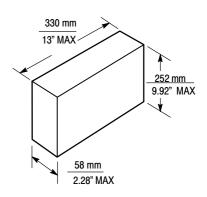
Figure 47. Fan Fold Box Dimensions
