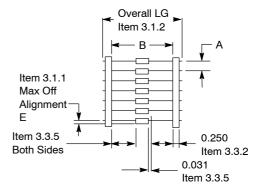
Figure 55. Component Spacing
