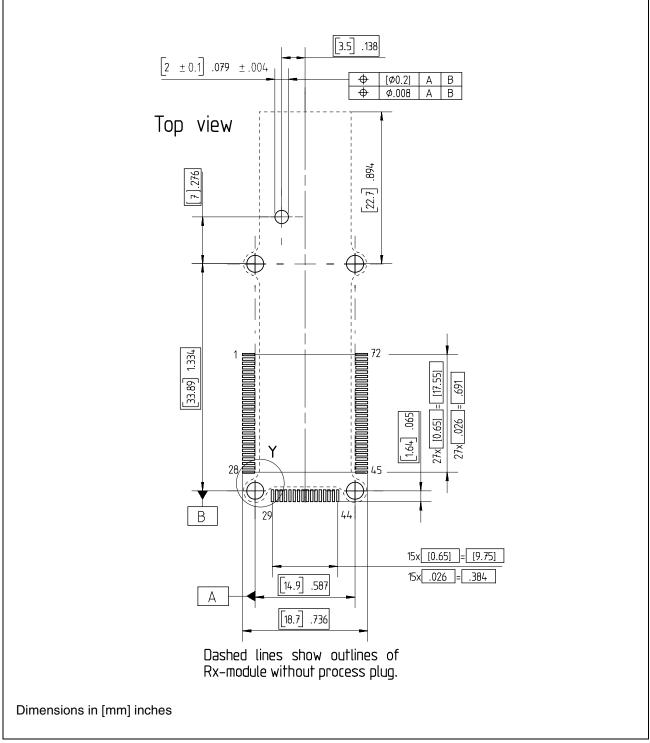
Figure 12Recommended Circuit Board Layout: Receiver
