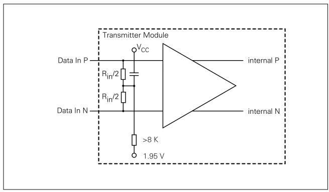
Figure 6 LVDS Input Stage
