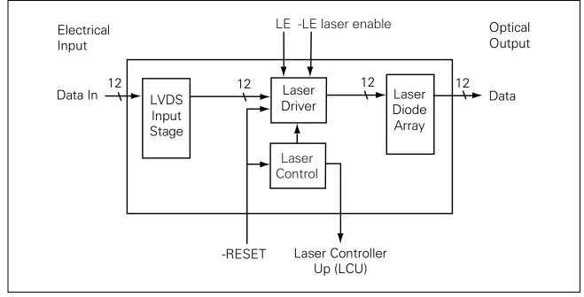
Figure 2 Transmitter Block Diagram
