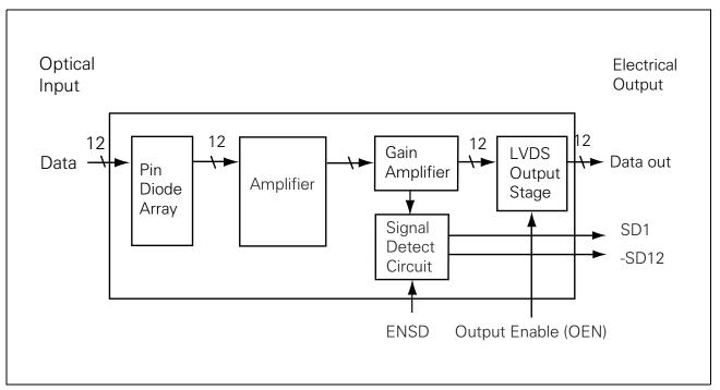
Figure 3 Receiver Block Diagram
