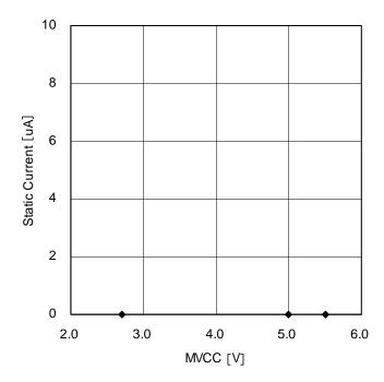
Figure 5. MVCC Static Current Voltage Dependency
