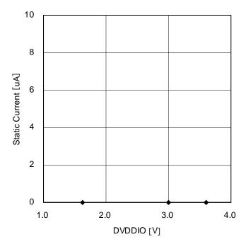
Figure 3. DVDDIO Static Current Voltage Dependency
