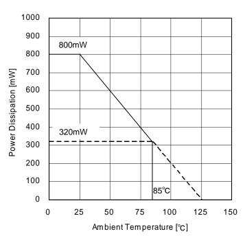
Figure 14. Power Dissipation Curve
