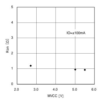
Figure 9. Output ON-Resistance
