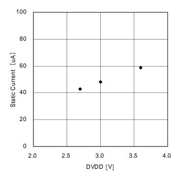
Figure 1. DVDD Static Current Voltage Dependency
