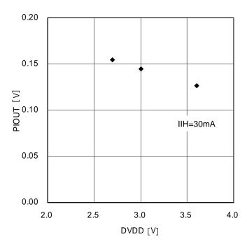
Figure 13. Output Voltage DVDD Dependency (PI driving circuit)
