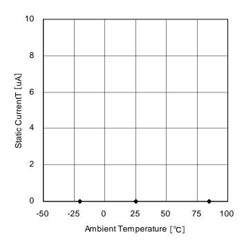
Figure 4. DVDDIO Static Current Temperature Dependency
