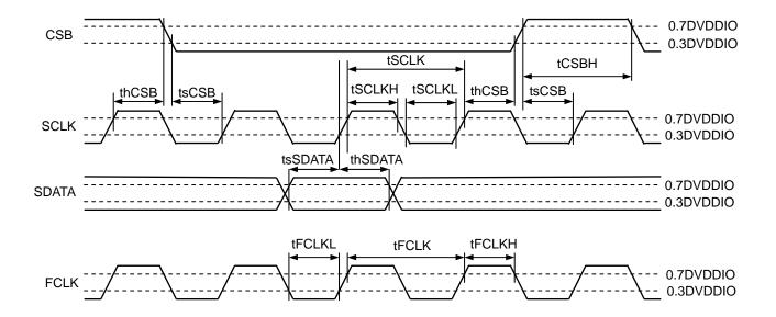
(note1) FCLK is asynchronous with SCLK. (note2) Duty of FCLK, SCLK are free.
