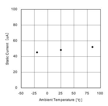
Figure 2. DVDD Static Current Temperature Dependency
