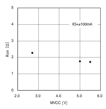
Figure 7. Output ON-Resistance MVCC Dependency (Voltage driver block)
