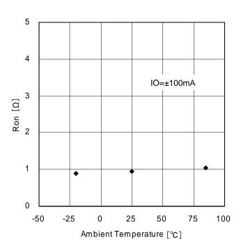
Figure 10. Output ON-Resistance
