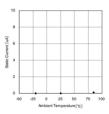
Figure 6. MVCC Static Current Temperature Dependency
