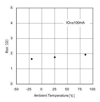
Figure 8. Output ON-Resistance
