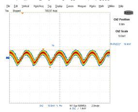
Fig. 20. Output Voltage Ripple, 3A load Ch<sub>2</sub>: V<sub>o</sub>
