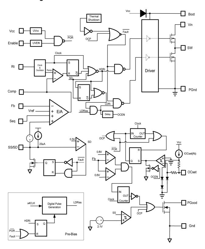
Fig. 2. Simplified block diagram of the IR3843A
