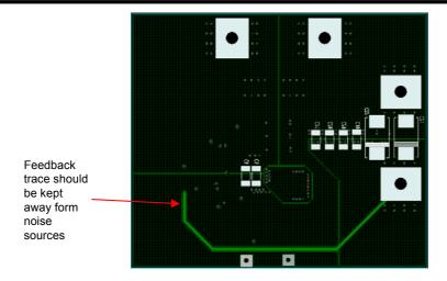
Fig. 26b. IRDC3843A demoboard layout considerations – Bottom Layer
