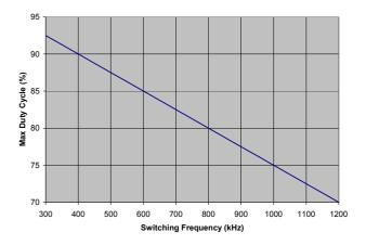
Fig. 10. Maximum duty cycle v/s switching frequency.
