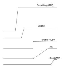
Fig. 3c. Recommended startup sequence, Sequenced operation
