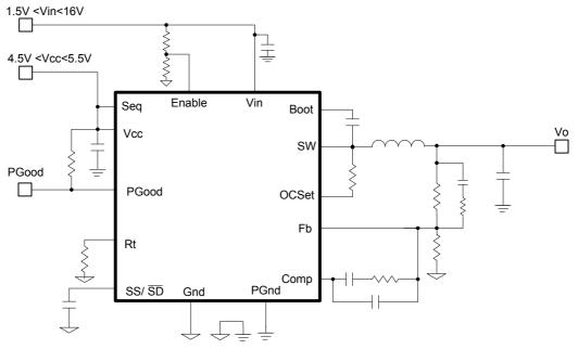
Fig. 1. Typical application diagram
