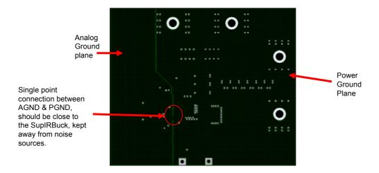
Fig. 26c. IRDC3843A demoboard layout considerations – Mid Layer 1
