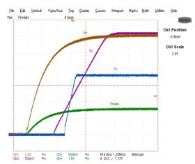
Fig. 17. Start up at 3A Load  $\mathrm{Ch_{1}:V_{in},\,Ch_{2}:V_{o},\,Ch_{3}:V_{ss},\,Ch_{4}:Enable}$
