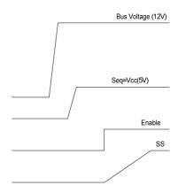
Fig. 3b. Recommended startup sequence, Non-Sequenced operation
