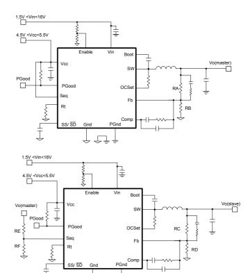
Fig. 8b. Application Circuit for Simultaneous Sequencing
