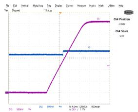
Fig. 19. Start up with 1.62V Pre Bias, 0A Load,  $\mathrm{Ch_2:V_0}$ ,  $\mathrm{Ch_3:V_{SS}}$
