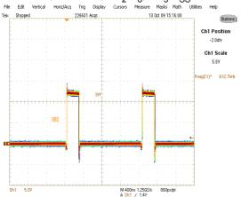
Fig. 21. Inductor node at 3A load Ch<sub>1</sub>:LX
