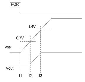
Fig. 6. Theoretical operation waveforms during soft-start
