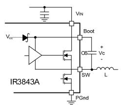
Fig. 12. Bootstrap circuit to generate Vc voltage
