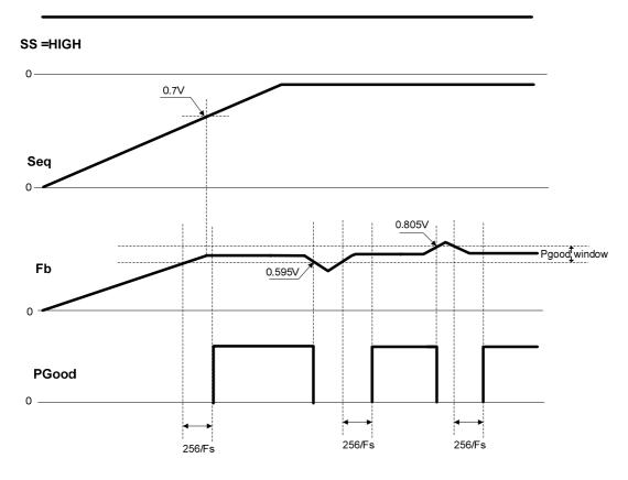
Fig.9b IR3843A Tracking Operation
