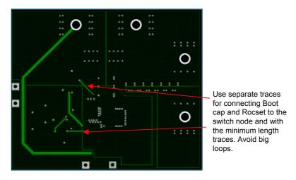
Fig. 26d. IRDC3843A demoboard layout considerations – Mid Layer 2
