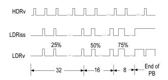
Fig. 5. Pre-Bias startup pulses
