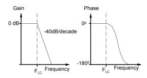
Fig. 13. Gain and Phase of LC filter
