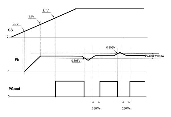
Fig.9a IR3843A Non-Tracking Operation (Seq=Vcc)
