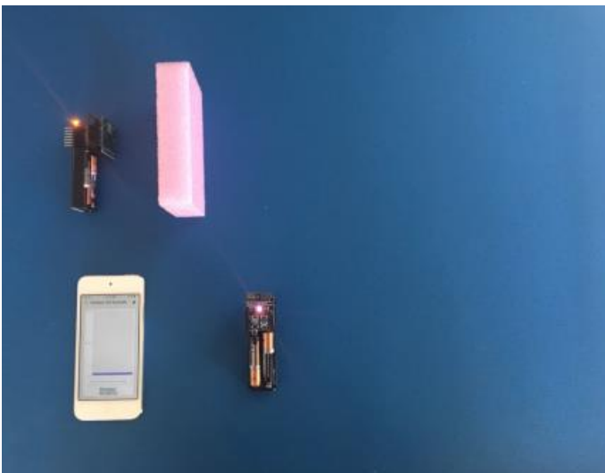
Figure 27 - ToF measurement with SimbleeForMobile and Paired Node - Short Distance
