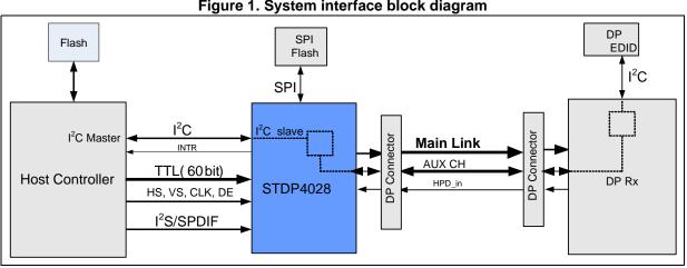
Figure 1. System interface block diagram
