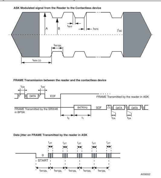
Figure 52. SRIX4K synchronous timing, transmit and receive
