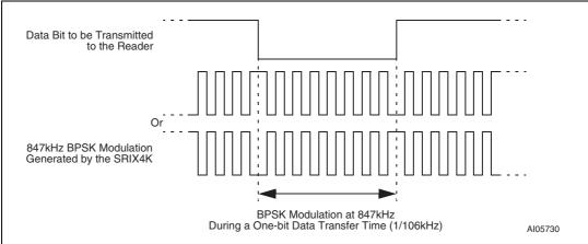
Figure 7. Wave transmitted using BPSK subcarrier modulation
