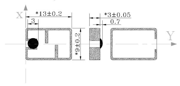
Mounting: The antenna is mounted with double sided adhesive tape that is attached to the antenna.
