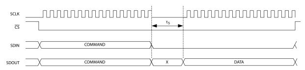
Figure 4-11: GSPI Read Timing – Single Read Access with Loop-Through Operation (default)
