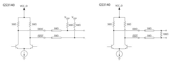
Figure 4-2: 50 $\Omega$  Termination to V<sub>TERM</sub>
