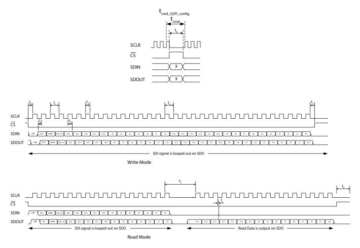
Figure 4-7: GSPI External Interface Timing
