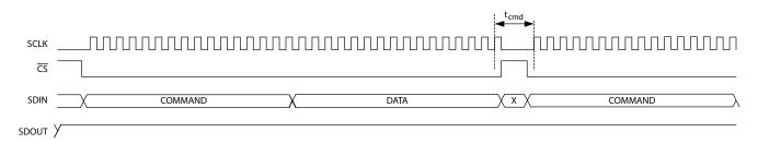
Figure 4-9: GSPI Write Timing – Single Write Access with GSPI Link-Disable Operation
