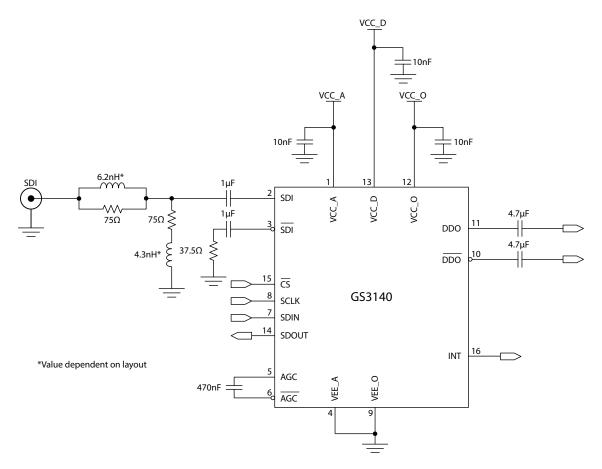
**Figure 6-1: Typical Application Circuit**
