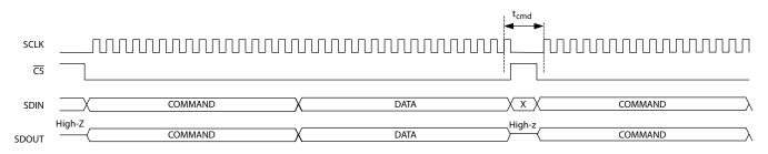
Figure 4-10: GSPI Write Timing – Single Write Access with Bus-Through Operation
