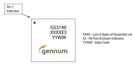
Figure 7-3: Marking Diagram
