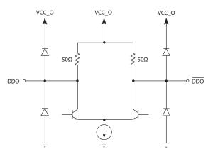
Figure 3-3: Serial Data Output
