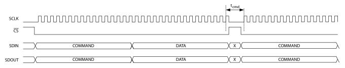
Figure 4-8: GSPI Write Timing – Single Write Access with Loop-Through Operation (default)
