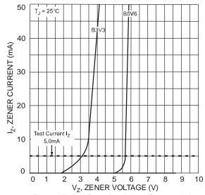
Figure 2 Typical Zener Breakdown Characteristics
