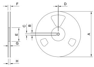
NOTE: Controlling dimensions in mm Std reel quantity is 4800 parts. (ordered as AUIRF7734M2TR). For 1000 parts on 7" reel, order AUIRF7734M2TR1
