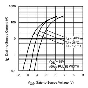
Fig 5. Typical Transfer Characteristics
