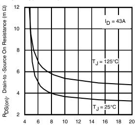
$\label{eq:VGS} \mbox{ V}_{\mbox{GS}, \mbox{ Gate -to -Source Voltage } (V) } \mbox{ Fig 3. Typical On-Resistance vs. Gate Voltage}$
