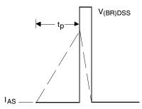
Fig 18b. Unclamped Inductive Waveforms
