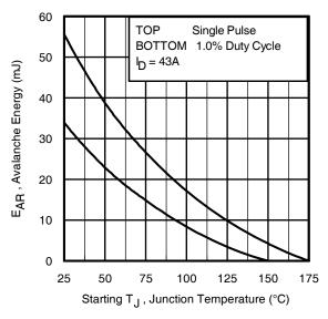
Fig 17. Maximum Avalanche Energy vs. Temperature
