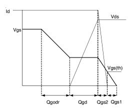
Fig 19b. Gate Charge Waveform
