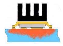
Mounted to a PCB with small clip heatsink (still air)
