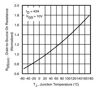
**Fig 6.** Normalized On-Resistance vs. Temperature www.irf.com
