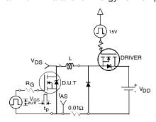
Fig 18a. Unclamped Inductive Test Circuit
