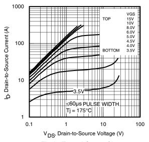
Fig 2. Typical Output Characteristics
