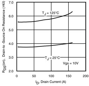
Fig 4. Typical On-Resistance vs. Drain Current
