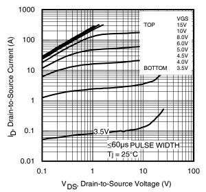
Fig 1. Typical Output Characteristics
