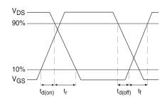
Fig 20b. Switching Time Waveforms
