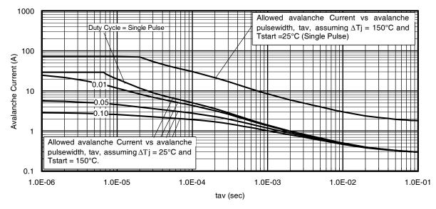
Fig 16. Typical Avalanche Current vs. Pulsewidth
