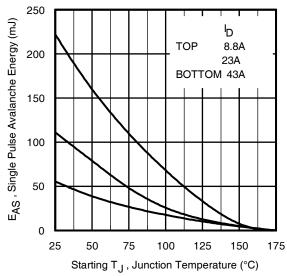
Fig 14. Maximum Avalanche Energy vs. Temperature
