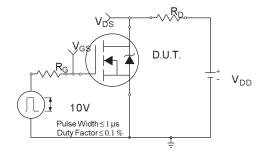
Fig 20a. Switching Time Test Circuit
