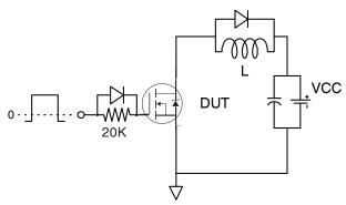
Fig 19a. Gate Charge Test Circuit
