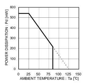
Reduce by 5.4mW/°C over 25°C. (70.0mm × 70.0mm × 1.6mm FR4 glass epoxy board)
