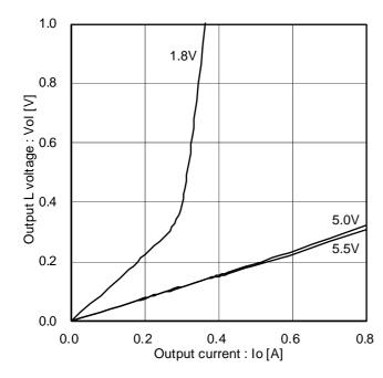
Figure 11. Output L voltage (Voltage characteristics)
