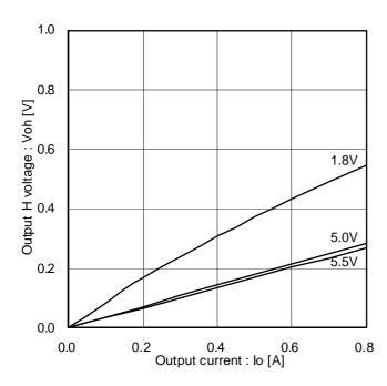
Figure 9. Output H voltage (Voltage characteristics)
