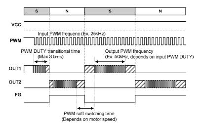
Figure 21. Timing chart in PWM control
