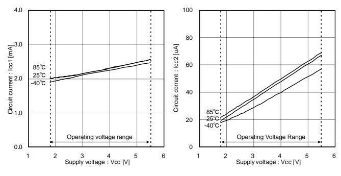
Figure 3. Circuit current 1
