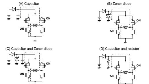
Figure 28. Measure against Vcc voltage rise
