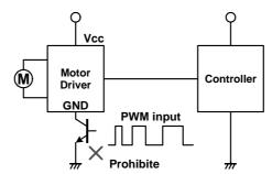
Figure 29. GND Line PWM switching prohibited
