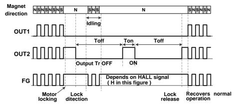
Figure 25. Lock protection timing chart
