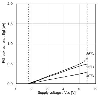
Figure 16. FG Output leak current
