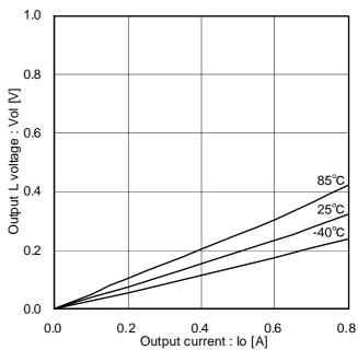
Figure 10. Output L voltage (Temperature characteristics)
