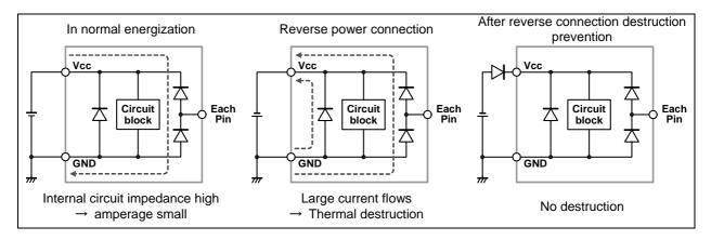
Figure 26. Flow of current when power is connected reversely
