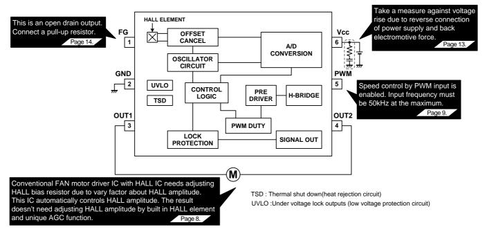
Figure 1. Block diagram and application circuit
