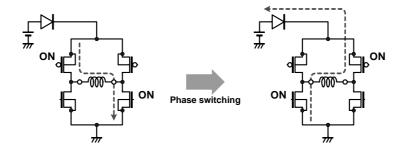
Figure 27. Vcc voltage rise by back electromotive force
