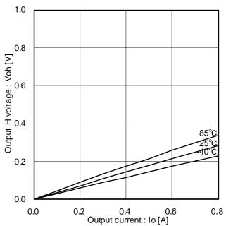
Figure 8. Output H voltage (Temperature characteristics)
