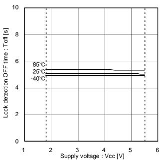
Figure 18. Lock detection OFF time
