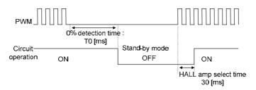
Figure 23. Stand-by mode and quick start function
