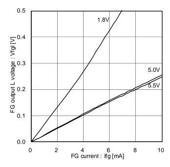
Figure 15. FG output L voltage (Voltage characteristics)
