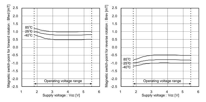
Figure 5. Magnetic switch-point for forward rotation
