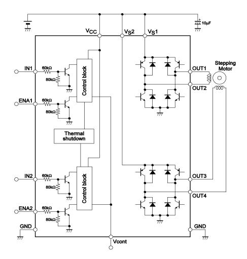
Note: As long as the voltages applied to V<sub>CC</sub>, V<sub>S</sub>1, V<sub>S</sub>2, ENA1, ENA2, IN1, and IN2 are within the limits set by the absolute maximum ratings, there are no restrictions on the relationship of each voltage level in comparison with the others (regarding which is higher or lower). (ex.  $V_{CC} = 3V$ ,  $V_{S}1$ , 2 = 2V, ENA = IN = 5V)
