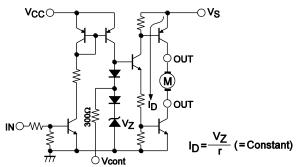
As shown in the left diagram, the Vcont pin outputs the voltage of the band gap Zener  $V_Z + V_F$  (= 1.93V). In normal use, this pin is left open.
