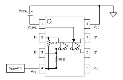
Figure 6. Standard Termination Method,  $V_{TT}$  Pin 4
