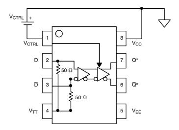
Figure 4. Voltage Source Implementation,  $V_{CTRL}$  Pin 1
