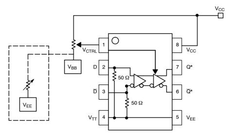
Figure 5. Alternative Implementations,  $V_{\text{CTRL}}$  Pin 1
