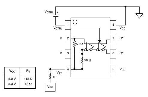
Figure 7. Alternate "Y" Termination Method, V<sub>TT</sub> Pin 4
