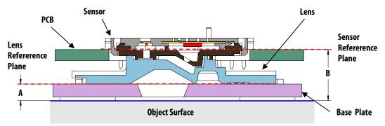
Figure 2. Optical system assembly cross-section diagram
