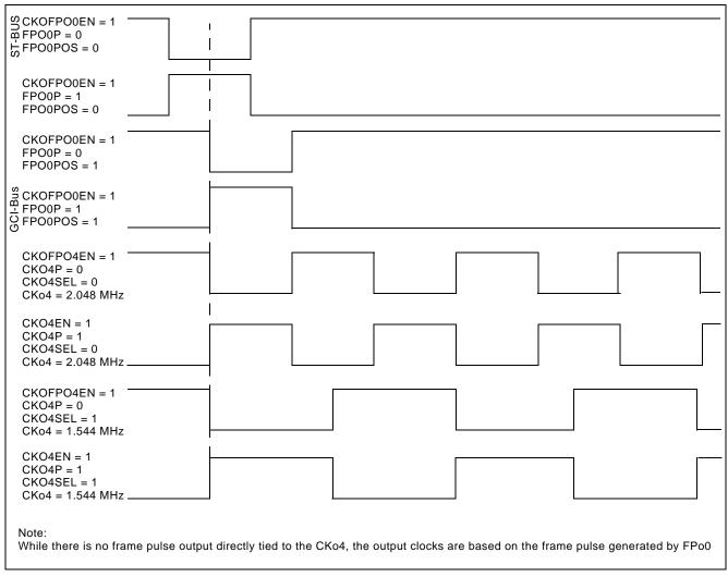
Figure 11 - Output Timing for CKo4
