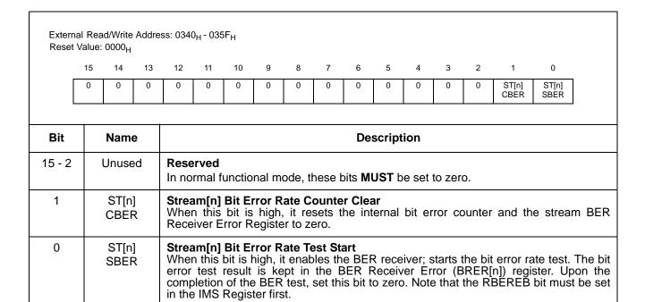
Table 50 - BER Receiver Control Register [n] (BRCR[n]) Bits
