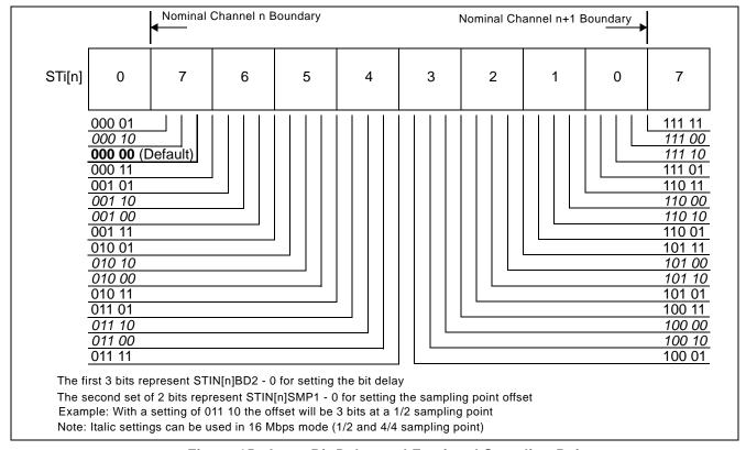
Figure 15 - Input Bit Delay and Factional Sampling Point
