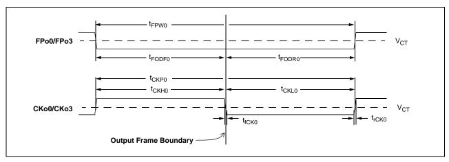
Figure 42 - FPo0 and CKo0 or FPo3 and CKo3 (4.096 MHz) Timing Diagram
