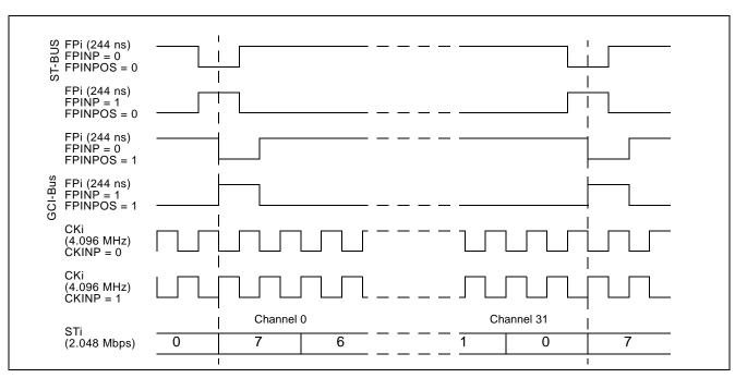
Figure 4 - Input Timing when CKIN1 - 0 bits = "10" in the CR
