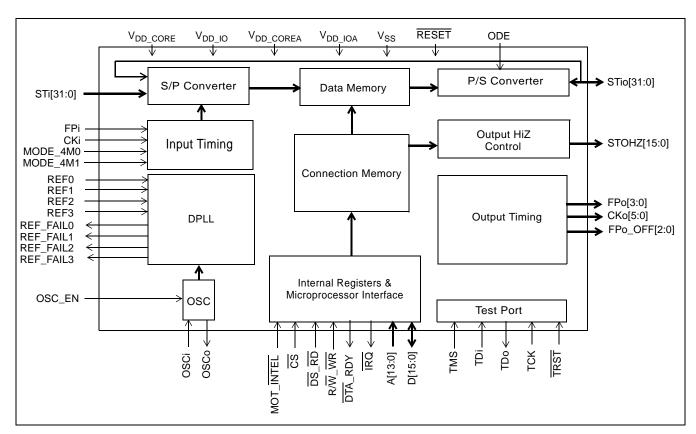
Figure 1 - ZL50022 Functional Block Diagram
