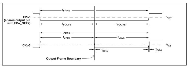
Figure 47 - CKo5 Timing Diagram (19.44 MHz)
