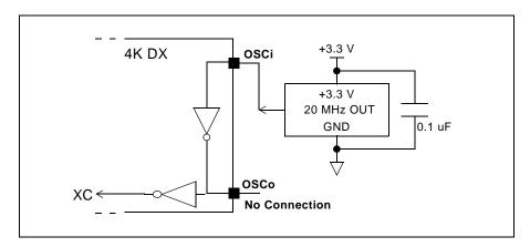
Figure 24 - Clock Oscillator Circuit
