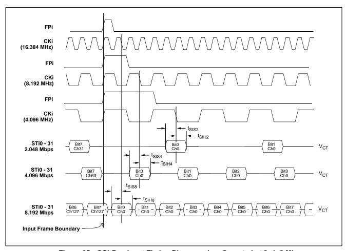
Figure 35 - GCI-Bus Input Timing Diagram when Operated at 2, 4, 8 Mbps
