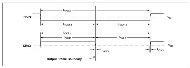
Figure 45 - FPo3 and CKo3 (32.768 MHz) Timing Diagram
