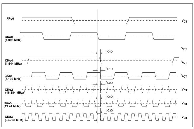
Figure 49 - Output Timing (ST-BUS Format)
