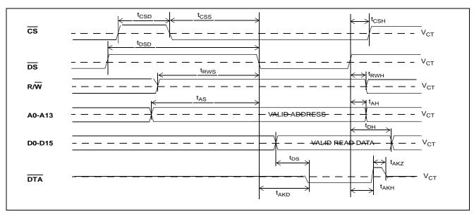
Figure 26 - Motorola Non-Multiplexed Bus Timing - Read Access
