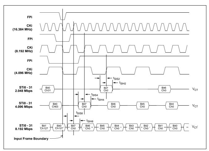
Figure 33 - ST-BUS Input Timing Diagram when Operated at 2, 4, 8 Mbps
