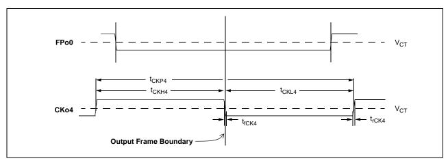
Figure 46 - FPo4 and CKo4 Timing Diagram (1.544/2.048 MHz)
