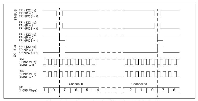
Figure 5 - Input Timing when CKIN1 - 0 bits = "01" in the CR
