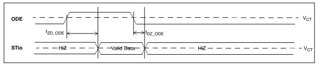
Figure 40 - Output Drive Enable (ODE)
