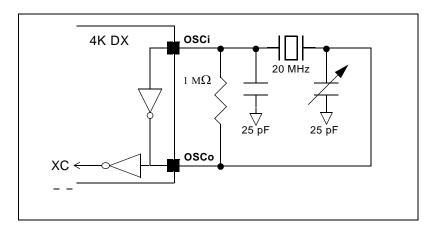
Figure 23 - Crystal Oscillator Circuit
