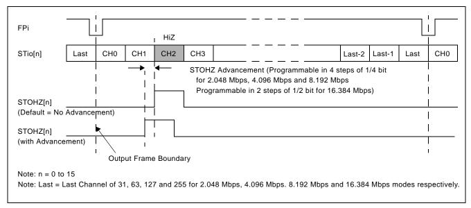
Figure 18 - Channel Switching External High Impedance Control Timing
