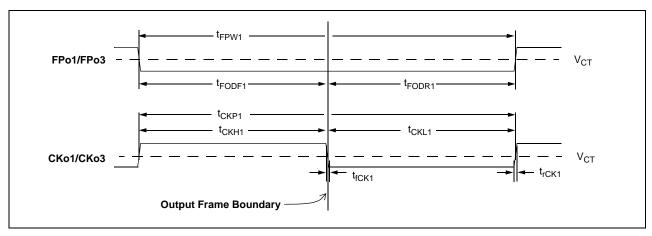
Figure 43 - FPo1 and CKo1 or FPo3 and CKo3 (8.192 MHz) Timing Diagram
