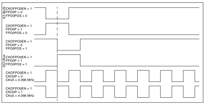
Figure 7 - Output Timing for CKo0 and FPo0
