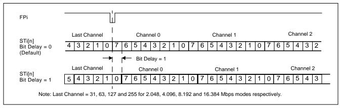
Figure 13 - Input Bit Delay Timing Diagram (ST-BUS)
