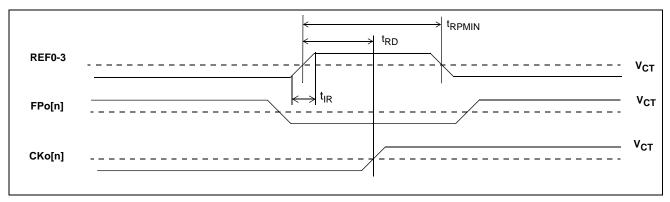
Figure 48 - REF0 - 3 Reference Input/Output Timing
