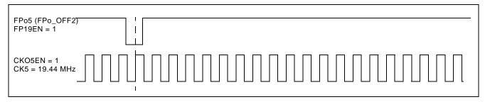
Figure 12 - Output Timing for CKo5 and FPo5 (FPo\_OFF2)
