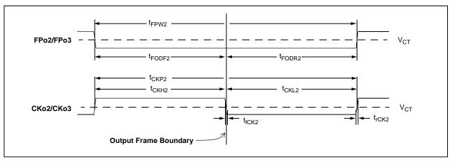
Figure 44 - FPo2 and CKo2 or FPo3 and CKo3 (16.384 MHz) Timing Diagram
