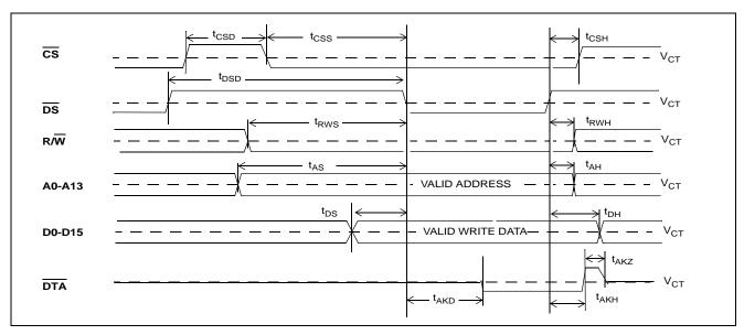
Figure 27 - Motorola Non-Multiplexed Bus Timing - Write Access
