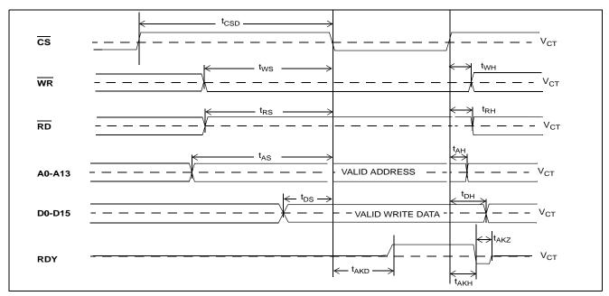
Figure 29 - Intel Non-Multiplexed Bus Timing - Write Access
