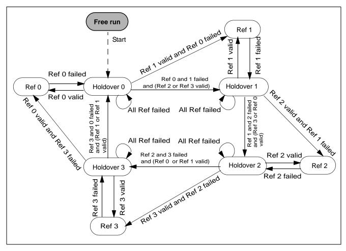
Figure 21 - Automatic Reference Switching State Diagram with No Preferred Reference
