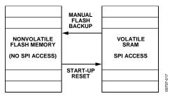
Figure 17. SRAM and Flash Memory Diagram
