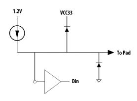
Figure 12. Low Speed IO Equivalent Circuit, RESETL
