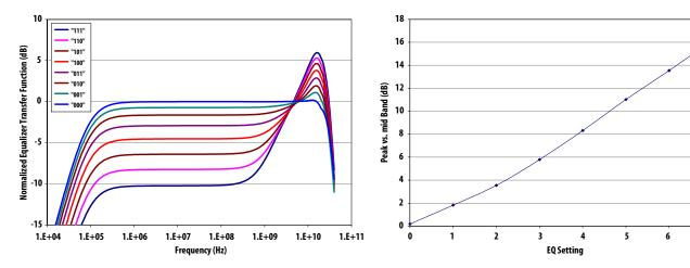
Figure 26. Normalized Equalization Transfer Function vs. Settings
