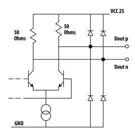
Figure 10. Receiver Data Output Equivalent Circuit
