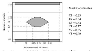
Transmitter eye mask definitions (TP2) at Hit ratio 5 x  $10^{-5}$  hits per sample
