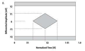
Rx Electrical Eye Mask Coordinates (TP4) at Hit ratio 5 x  $10^{-5}$  hits per sample
