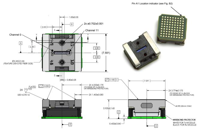
Figure A1. Module Top and Side View
