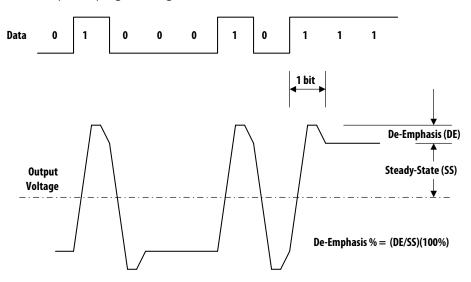
Figure 5. Definition of De-emphasis and Steady State
