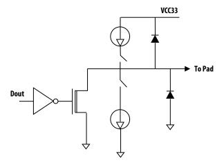
Figure 11. Low Speed IO Equivalent Circuit, INTL
