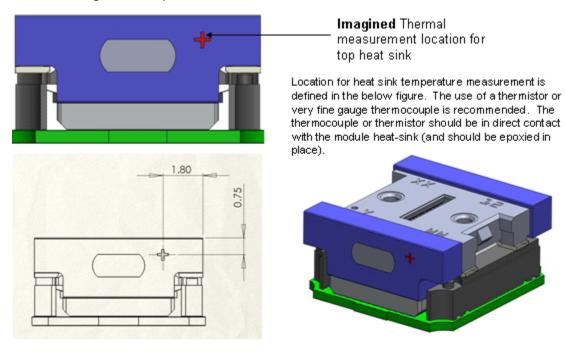
Figure 22. Module Thermal Interface (RX shown)
