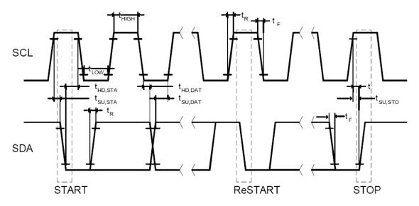
Figure 24. 2-wire Serial Interface Timing Diagram
