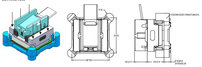
Figure 21. A Module and PRIZM in a Reference LGA Socket
