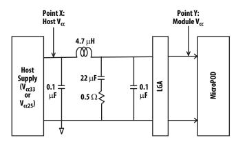
Figure 8. Recommended TX and RX Power Supply Filter
