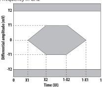
Tx Electrical Eye Mask Coordinates (TP1a) at Hit ratio 5 x 10<sup>-5</sup> hits per sample
