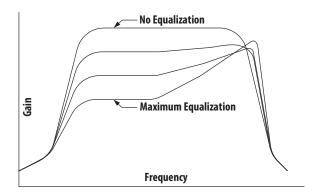
**Figure 4. Transmitter Input Equalization**
