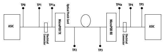
Figure 6. Link Model test point definitions
