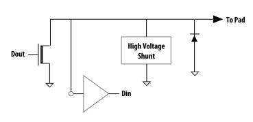
Figure 14. Low Speed IO Equivalent Circuit, SDA, SCL
