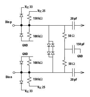
Figure 9. Transmitter Data Input Equivalent Circuit
