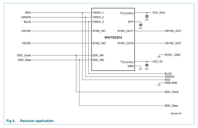
The receiver application simplifies VGA input circuit applications.
