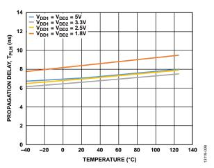
Figure 8. Propagation Delay, T<sub>PLH</sub> vs. Temperature at Various Voltages
