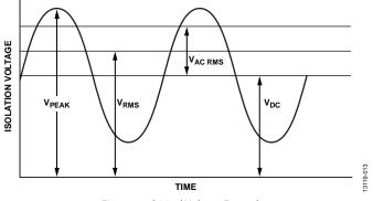
Figure 15. Critical Voltage Example
