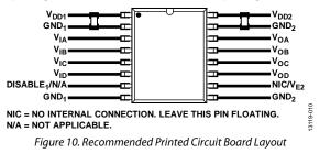
In applications involving high common-mode transients, ensure that board coupling across the isolation barrier is minimized. Furthermore, design the board layout such that any coupling that does occur equally affects all pins on a given component side. Failure to ensure this can cause voltage differentials between pins exceeding the Absolute Maximum Ratings of the device, thereby leading to latch-up or permanent damage.
