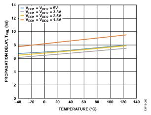
Figure 9. Propagation Delay, T<sub>PHL</sub> vs. Temperature at Various Voltages
