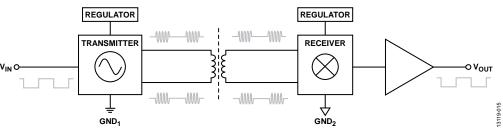
Figure 12. Operational Block Diagram of a Single Channel with a High Fail-Safe Output State
