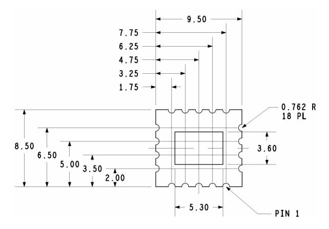
The nominal size of the part is 8.5x9.5mm with a height of 1.3 mm
