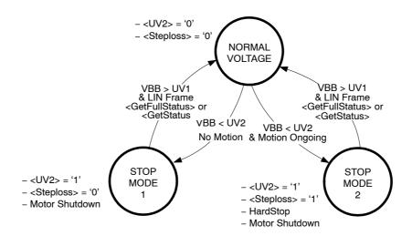
Figure 16. State Diagram Battery Voltage Management
