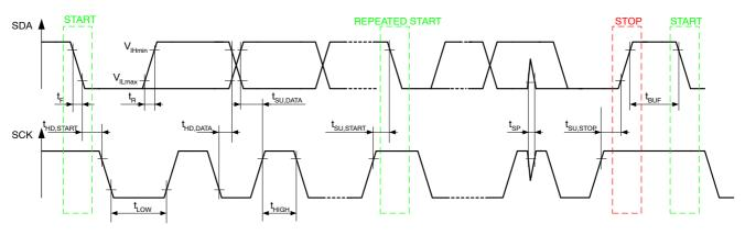
Figure 5. I<sup>2</sup>C Timing Diagrams
