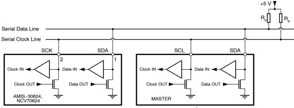
Figure 22. Connection of a Device to the I<sup>2</sup>C-bus
