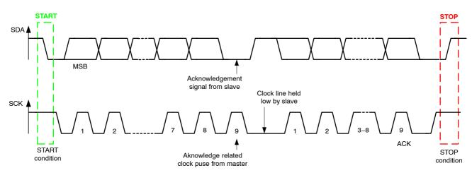
Figure 25. Data Transfer on the I<sup>2</sup>C-bus
