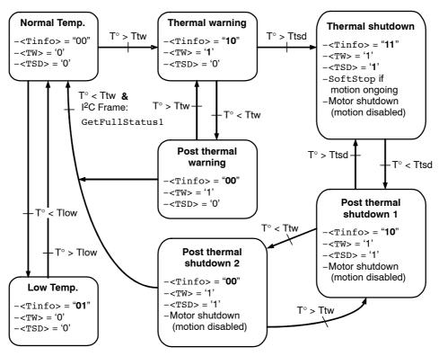
Figure 14. State Diagram Temperature Management
