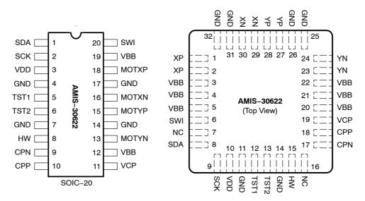
Figure 2. SOIC-20 and NQFP-32 Pin-out
