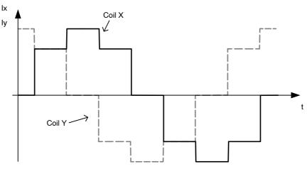
Figure 18. Current Waveforms in Motor Coils X and Y in Halfstep Mode
