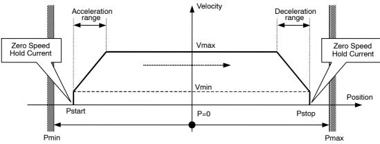
Figure 7. Positioning and Motion Control
