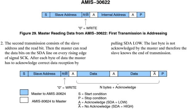
Figure 30. Master Reading Data from AMIS-30622: Second Transmission is Reading Data
