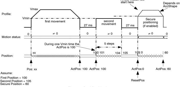
Figure 8. Dual Positioning
