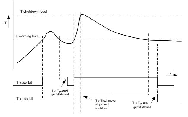
Figure 15. Illustration of Thermal Management Situation
