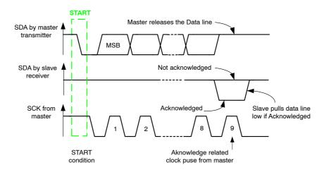
Figure 26. Acknowledge on the I<sup>2</sup>C-bus
