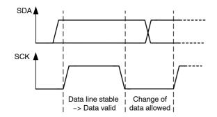
Figure 23. Bit Transfer on the I<sup>2</sup>C-bus
