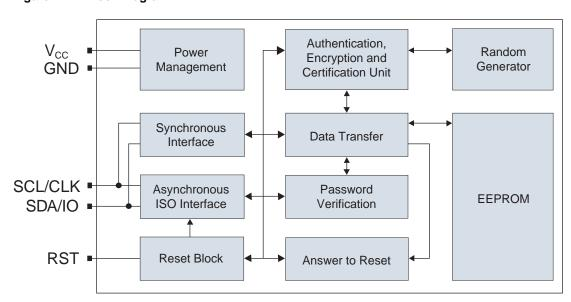
Figure 1-1. Block Diagram
