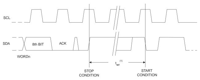
Note: The write cycle time  $t_{WR}$  is the time from a valid stop condition of a write sequence to the end of the internal clear/write cycle
