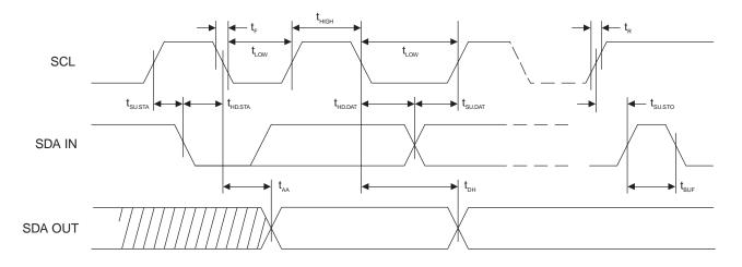
Figure 5-2. Write Cycle Timing
