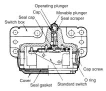
Apply extra tightening to the cap screw on the conduit.
