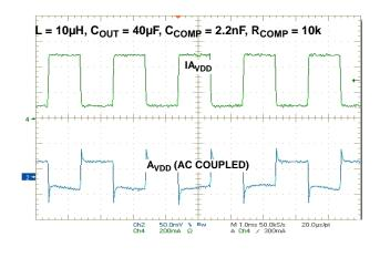
FIGURE 4. BOOST CONVERTER TRANSIENT RESPONSE
