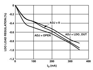
FIGURE 6. LDO LOAD REGULATION vs IO
