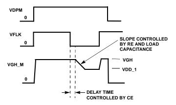
FIGURE 17. GATE PULSE MODULATOR TIMING DIAGRAM
