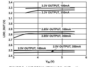
FIGURE 5. LINE REGULATION LDO\_OUT vs  $\rm V_{IN}$
