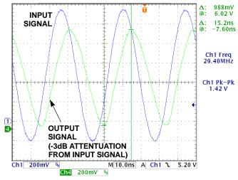
FIGURE 12.  $V_{\text{COM}}$  BANDWIDTH MEASUREMENT
