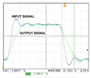
FIGURE 11.  $V_{\text{COM}}$  RISING SLEW RATE
