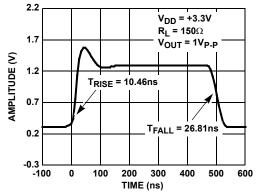
FIGURE 11. LARGE SIGNAL STEP RESPONSE
