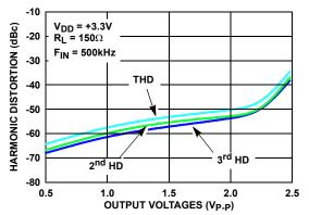
FIGURE 16. HARMONIC DISTORTION vs OUTPUT VOLTAGE
