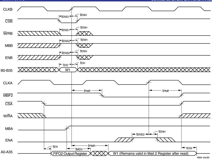
1. If Port B is configured for word size, data can be written to the Mail2 Register using B0-B17 (B18-B35 are don't care inputs). In this first case A0-A17 will have valid data (A18-A35 will be indeterminate). If Port B is configured for byte size, data can be written to the Mail2 Register using B0-B8 (B9-B35 are don't care inputs). In this second case, A0-A8 will have valid data (A9-A35 will be indeterminate).
