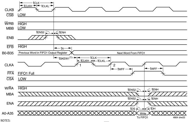
1. tskEw1 is the minimum time between a rising CLKB edge and a rising CLKA edge for FFA to transition HIGH in the next CLKA cycle. If the time between the rising CLKB edge and rising CLKA edge is less than tskEw1, then FFA may transition HIGH one CLKA cycle later than shown.
