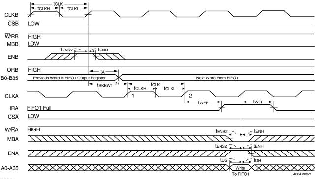
2. If Port B size is word or byte, tskew1 is referenced to the rising CLKB edge that reads the last word or byte write of the long word, respectively.
