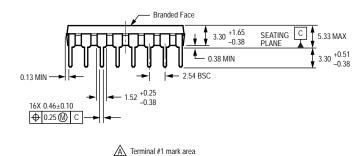
For Reference Only; not for tooling use (reference MS-001BB) Dimensions in millimeters Dimensions exclusive of mold flash, gate burrs, and dambar protrusions Exact case and lead configuration at supplier discretion within limits shown
