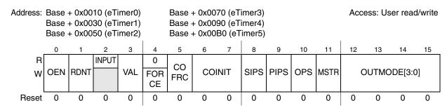
Figure 26-11. Control register 2 (CTRL2)
