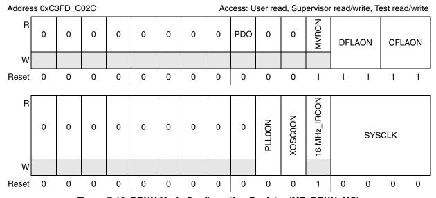
Figure 7-12. DRUN Mode Configuration Register (ME\_DRUN\_MC)
