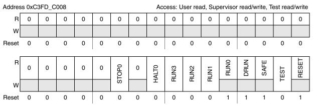
Figure 7-4. Mode Enable Register (ME\_ME)
