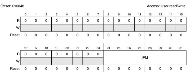
Figure 21-24. Identifier filter mode register (IFMR)
