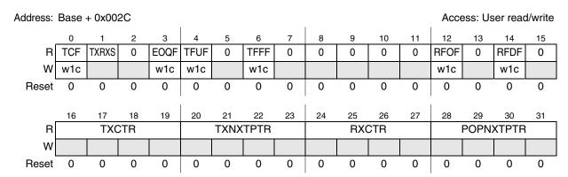
Figure 20-6. DSPI Status Register (DSPIx\_SR)
