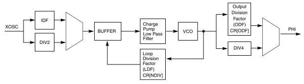
Figure 4-6. FMPLL block diagram
