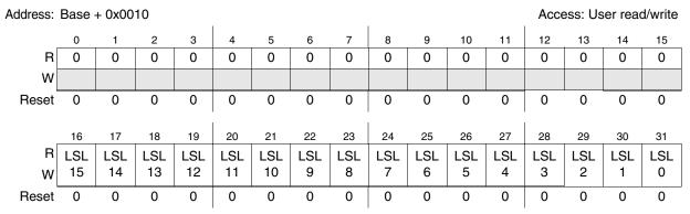
Figure 17-15. Low/Mid Address Space Block Select register (LMS)
