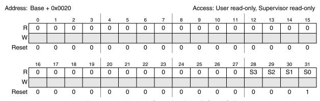
Figure 28-11. Module State Register (FCU\_MSR)
