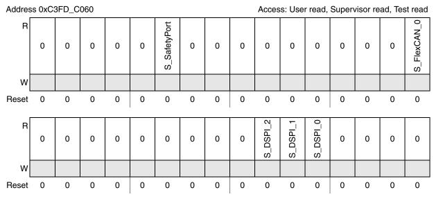
Figure 7-16. Peripheral Status Register 0 (ME\_PS0)
