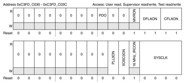
Figure 7-13. RUN0...3 Mode Configuration Registers (ME\_RUN0...3\_MC)
