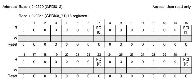
Figure 11-13. GPIO Pad Data Input registers 0\_3-68\_71 (GPDI[0\_3:68\_71])
