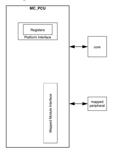
Figure 6-1. MC\_PCU Block Diagram
