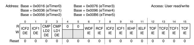
Figure 26-14. Interrupt and DMA enable register (INTDMA)
