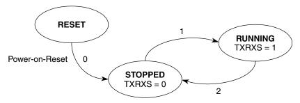
Figure 20-13. DSPI start and stop state diagram
