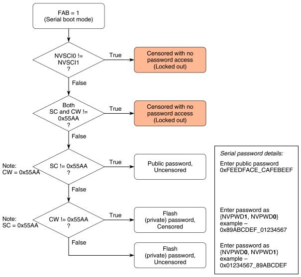
Figure 33-16. Censorship control in serial boot mode
