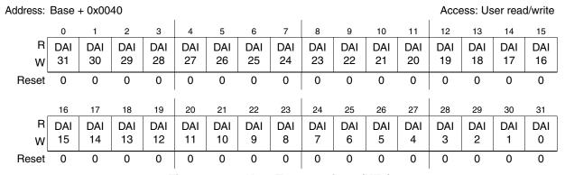
Figure 17-21. User Test 1 register (UT1)
