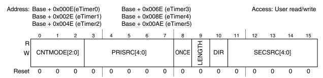
Figure 26-10. Control register 1 (CTRL1)
