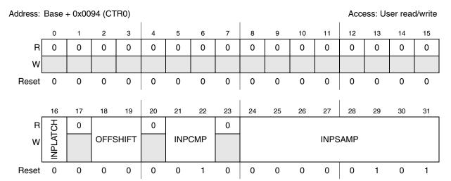
Figure 23-18. Conversion Timing Registers CTR[0]
