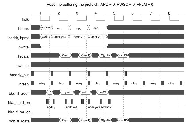
Figure 17-2. 1-cycle access, no buffering, no prefetch
