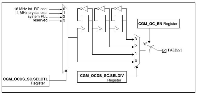
Figure 5-16. MC CGM Output Clock Multiplexer and PAD[22] Generation
