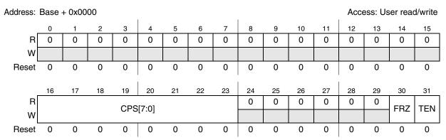
Figure 31-1. STM Control Register (STM\_CR)
