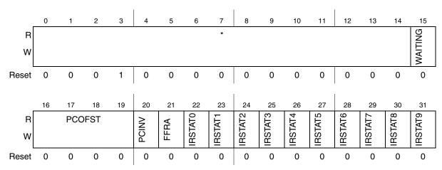
Figure 36-17. Control State Register (CTL)
