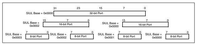
Figure 11-19. Data port example arrangement showing configuration for different port width accesses
