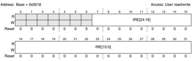
Figure 11-6. Interrupt Request Enable Register (IRER)
