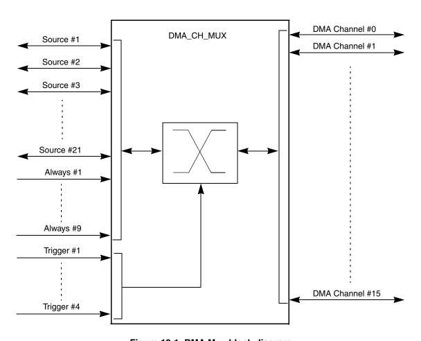
Figure 19-1. DMA Mux block diagram
