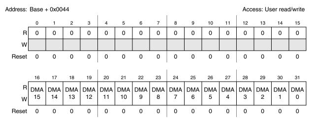
Figure 23-15. DMA Channel Select Register 0 (DMAR0)
