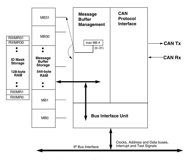
Figure 22-1. FlexCAN block diagram
