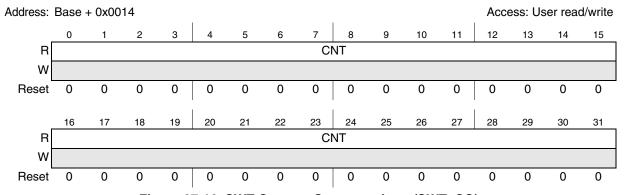
Figure 27-16. SWT Counter Output register (SWT\_CO)
