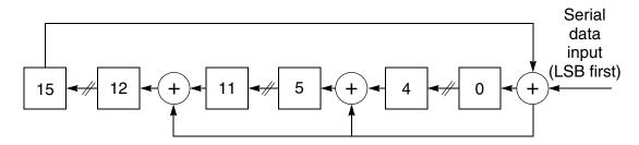
Figure 32-2. CRC-CCITT engine concept scheme
