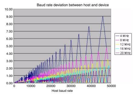
Figure 33-12. Baud rate deviation between host and MPC5602P
