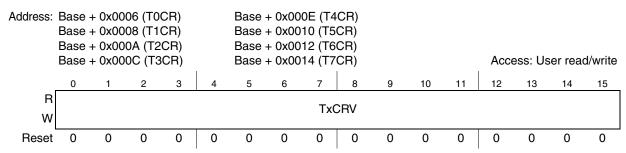
Figure 24-11. Trigger x Compare Register (TxCR, x = 0...7)
