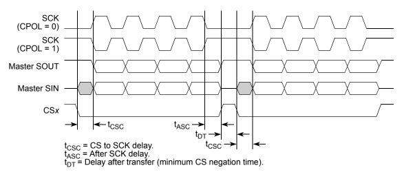
Figure 20-20. Example of non-continuous format (CPHA = 1, CONT = 0)
