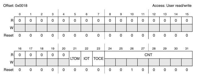
Figure 21-12. LIN timeout control status register (LINTCSR)
