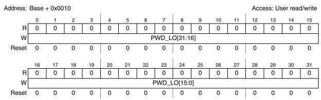
Figure 10-8. Password Comparison Register Low Word (PWCMPL) register
