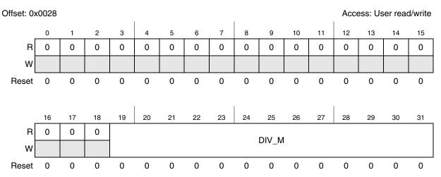
Figure 21-16. LIN integer baud rate register (LINIBRR)
