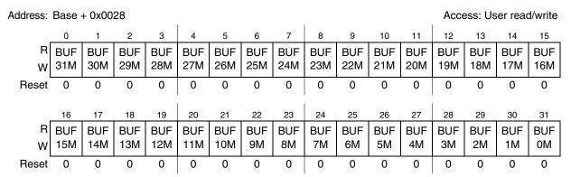
Figure 22-12. Interrupt Masks 1 Register (IMASK1)
