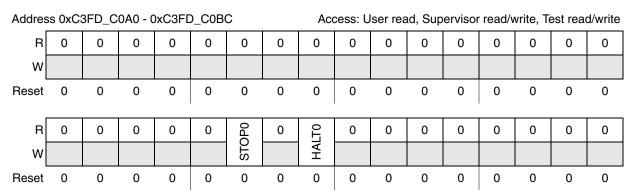
Figure 7-20. Low-Power Peripheral Configuration Registers (ME\_LP\_PC0...7)
