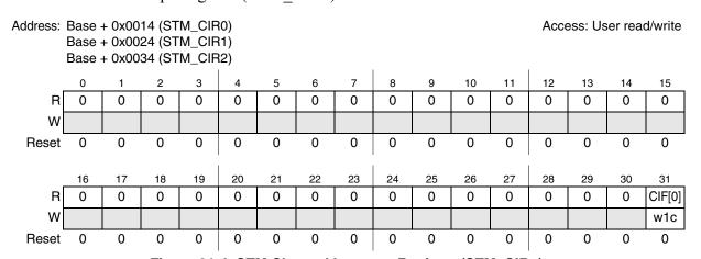
Figure 31-4. STM Channel Interrupt Register (STM\_CIRn)
