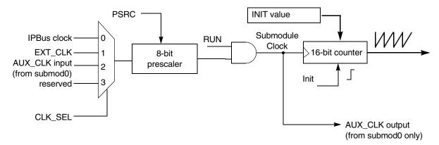
Figure 25-37. Clocking block diagram for each PWM submodule
