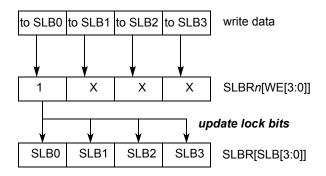
Figure 27-7. Change lock settings for 32-bit protected addresses
