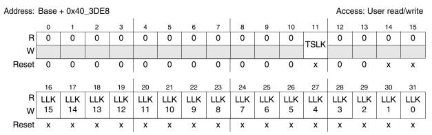
Figure 17-12. Non-Volatile Low/Mid Address Space Block Locking register (NVLML)
