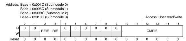
Figure 25-15. Interrupt Enable register (INTEN)
