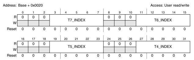
Figure 24-15. Commands list control register 2 (CLCR2)
