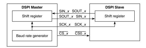
Figure 20-12. SPI serial protocol overview
