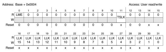
Figure 17-11. Low/Mid Address Space Block Locking register (LML)
