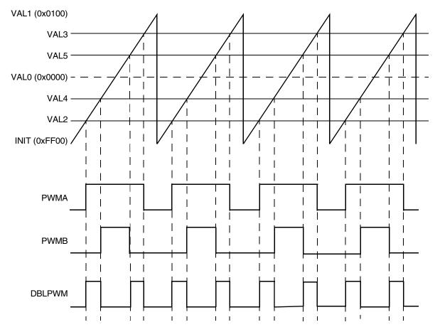
Figure 25-33. Double switching output example
