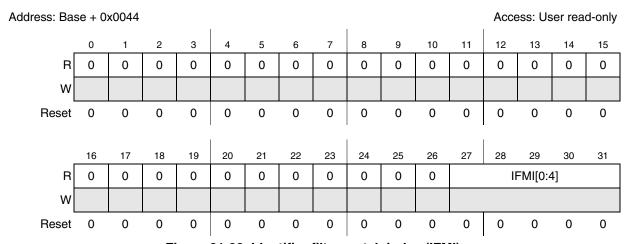
Figure 21-23. Identifier filter match index (IFMI)
