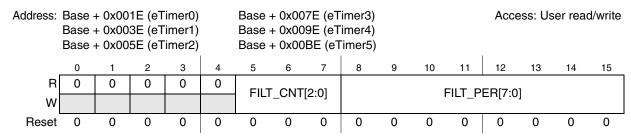
Figure 26-18. Input Filter register (FILT)
