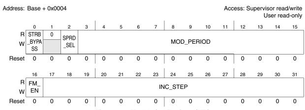
Figure 4-8. Modulation Register (MR)
