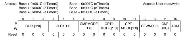
Figure 26-17. Compare and Capture Control register (CCCTRL)
