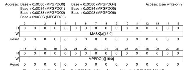
Figure 11-16. Masked Parallel GPIO Pad Data Out register 0-6 (MPGPDO[0:6])
