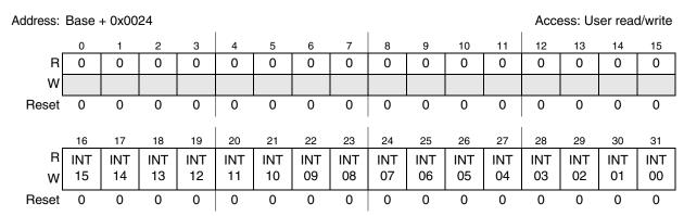
Figure 18-14. eDMA Interrupt Request Low Register (EDMA\_IRQRL)
