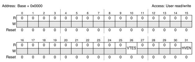
Figure 9-2. INTC Module Configuration Register (INTC\_MCR)
