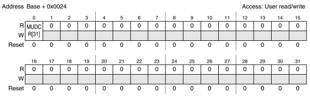
Figure 15-8. Miscellaneous User-Defined Control register (MUDCR)
