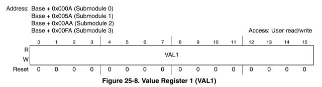
The 16-bit signed value written to this register defines the modulo count value (maximum count) for the submodule counter. Upon reaching this count value, the counter will reload itself with the contents of the INIT register. This register is not byte accessible.
