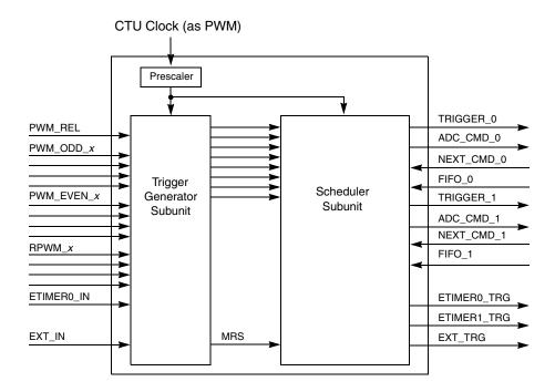
Figure 24-1. Cross triggering unit diagram
