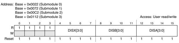
Figure 25-18. Fault Disable Mapping register (DISMAP)
