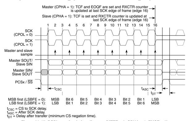
Figure 20-17. DSPI transfer timing diagram (MTFE = 0, CPHA = 1, FMSZ = 8)
