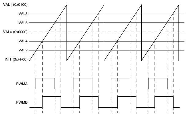
Figure 25-31. Phase-shifted outputs example
