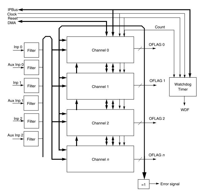
Figure 26-1. eTimer block diagram
