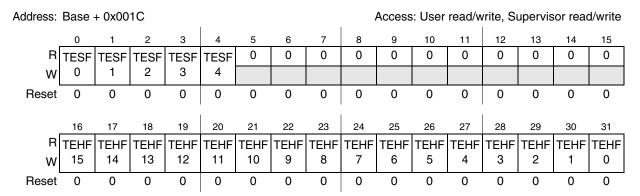
Figure 28-10. Timeout Enable Register (FCU\_TER)
