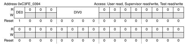
Figure 5-11. Auxiliary Clock 2 Divider Configuration Register (CGM\_AC2\_DC0)
