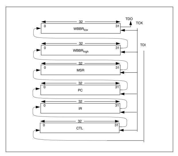
Figure 36-16. CPU Scan Chain Register (CPUSCR)
