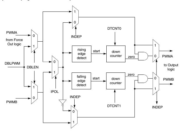
Figure 25-44. Deadtime insertion and fine control logic
