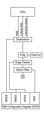
Figure 29-3. NMI pad diagram
