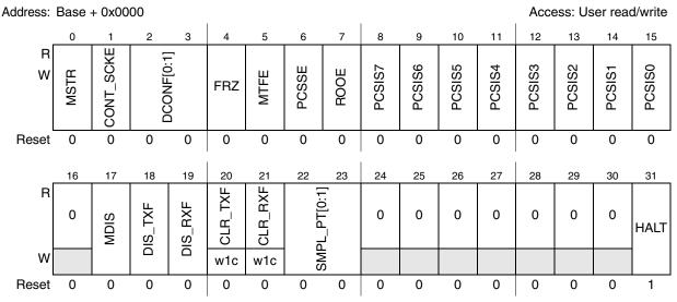
Figure 20-3. DSPI Module Configuration Register (DSPIx\_MCR)
