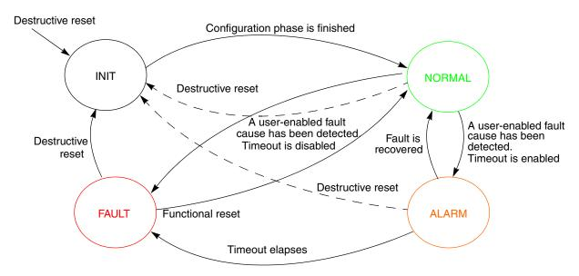
Figure 28-15. Finite state machine
