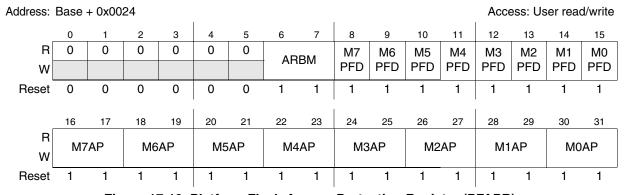
Figure 17-19. Platform Flash Access Protection Register (PFAPR)
