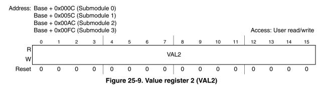
The 16-bit signed value in this register defines the count value to set PWMA high (Figure 25-2). This register is not byte accessible.
