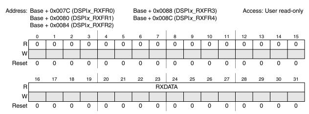
Figure 20-11. DSPI Receive FIFO Registers 0–4 (DSPIx\_RXFRn)
