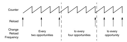
Figure 25-54. Full cycle reload frequency change
