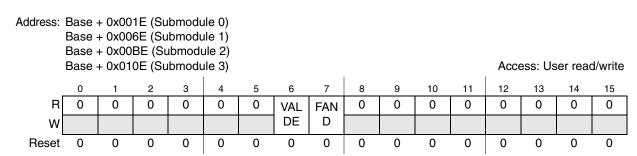
Figure 25-16. DMA Enable register (DMAEN)
