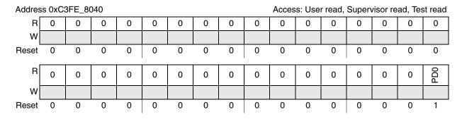
Figure 6-2. Power Domain Status Register (PCU\_PSTAT)
