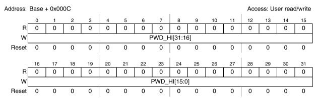
Figure 10-7. Password Comparison Register High Word (PWCMPH) register
