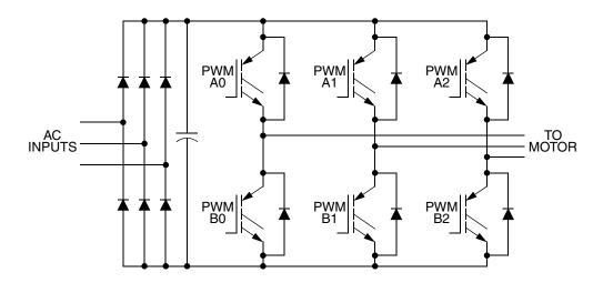
Figure 25-43. Typical 3-phase AC motor drive
