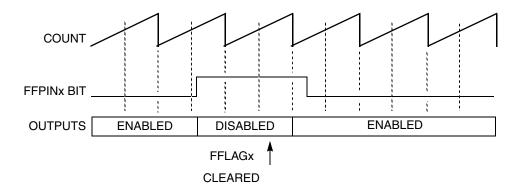
Figure 25-52. Manual fault clearing (FSAFE = 0)
