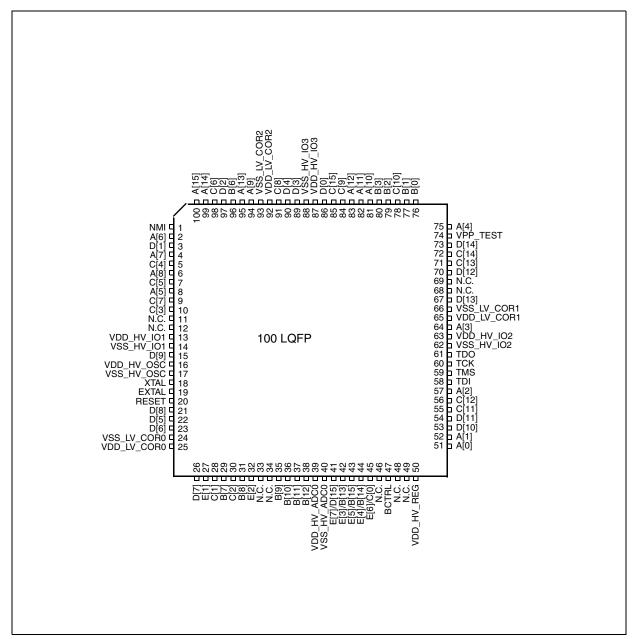
Figure 3-1. 100-pin LQFP pinout (top view)
