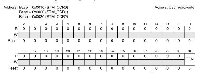
Figure 31-3. STM Channel Control Register (STM\_CCRn)
