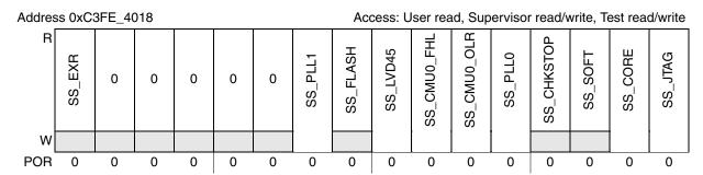
Figure 8-7. Functional Event Short Sequence Register (RGM\_FESS)
