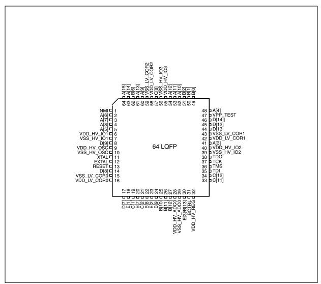
Figure 3-2. 64-pin LQFP pinout(top view)
