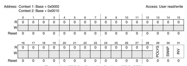
Figure 32-4. CRC Configuration Register (CRC\_CFG)
