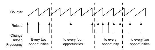
Figure 25-56. Full and half cycle reload frequency change
