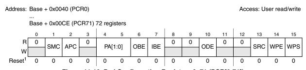
Figure 11-10. Pad Configuration Registers 0-71 (PCR[0:71])
