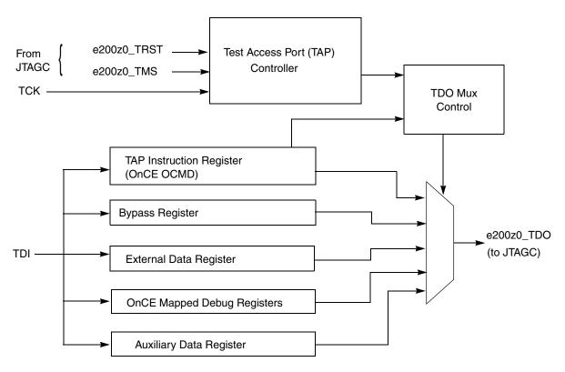
Figure 35-6. e200z0 OnCE block diagram
