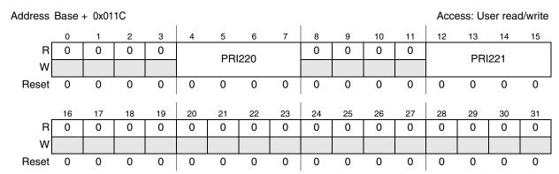
Figure 9-9. INTC Priority Select Register 220-221 (INTC\_PSR[220:221])
