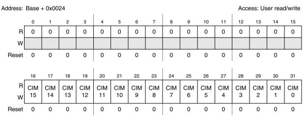
Figure 23-11. Channel Interrupt Mask Register 0 (CIMR0)
