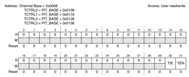
Figure 30-5. Timer Control register *n* (TCTRL*n*)
