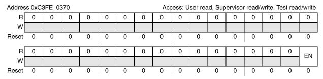
Figure 5-2. Output Clock Enable Register (CGM\_OC\_EN)
