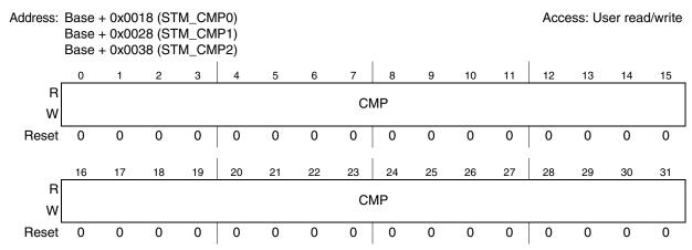
Figure 31-5. STM Channel Compare Register (STM\_CMPn)
