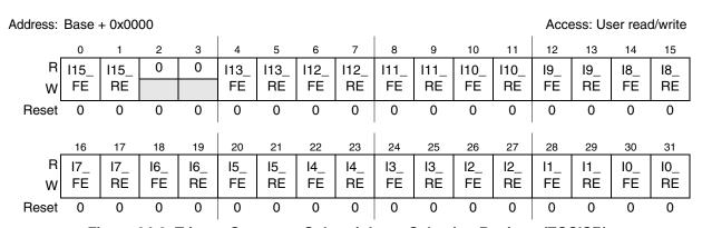
Figure 24-9. Trigger Generator Sub-unit Input Selection Register (TGSISR)
