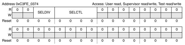
Figure 5-3. Output Clock Division Select Register (CGM\_OCDS\_SC)
