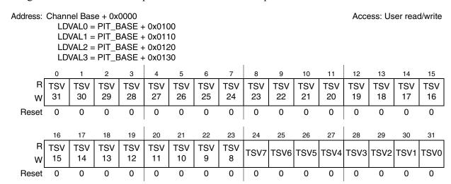
Figure 30-3. Timer Load Value Register n (LDVALn)
