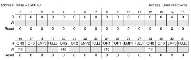
Figure 24-23. FIFO status register (FST)
