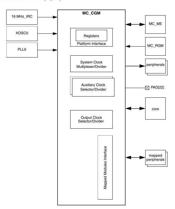
Figure 5-1. MC\_CGMBlock Diagram
