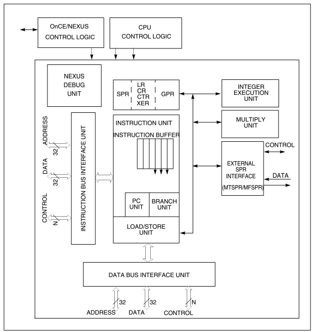
Figure 12-2. e200z0h block diagram
