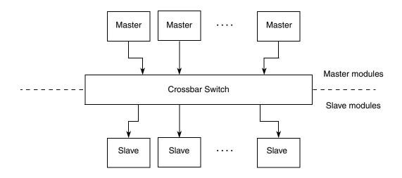
Figure 14-1. XBAR block diagram
