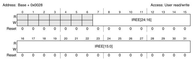
Figure 11-7. Interrupt Rising-Edge Event Enable Register (IREER)
