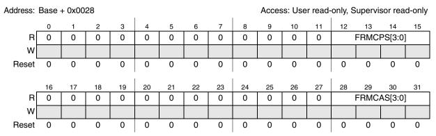
Figure 28-13. Frozen MC State Register (FCU\_FMCSR)
