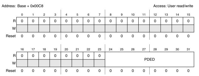
Figure 23-21. Power-Down Exit Delay Register (PDEDR)
