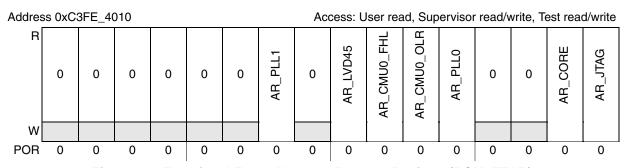
Figure 8-6. Functional Event Alternate Request Register (RGM\_FEAR)
