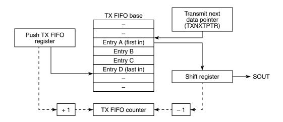
Figure 20-25. TX FIFO pointers and counter
