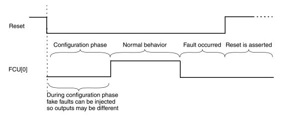
Figure 28-18. Bi-stable coding example
