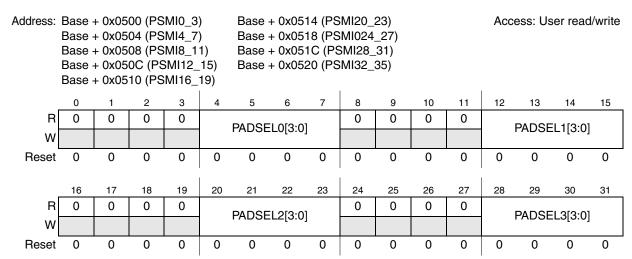
Figure 11-11. Pad Selection for Multiplexed Inputs registers (PSMI[0\_3:32\_35])
