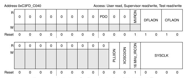
Figure 7-14. HALTO Mode Configuration Register (ME\_HALTO\_MC)
