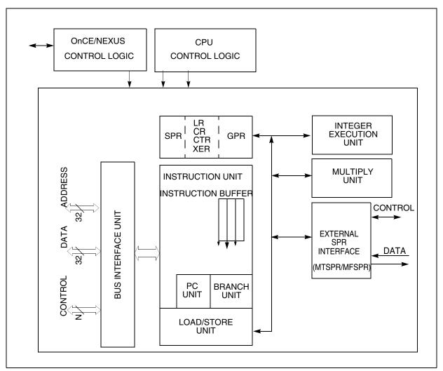
Figure 12-1. e200z0 block diagram
