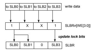
Figure 27-8. Change lock settings for mixed protection
