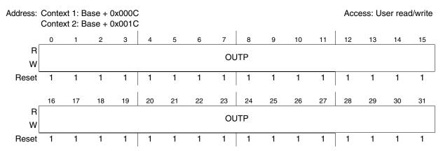
Figure 32-7. CRC Output Register (CRC\_OUTP)
