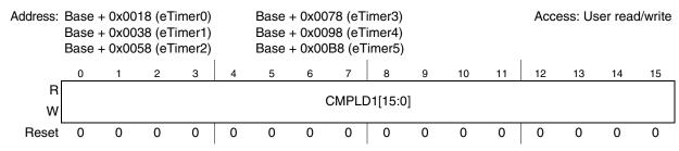
Figure 26-15. Comparator Load 1 (CMPLD1)
