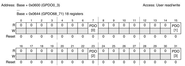
Figure 11-12. Port GPIO Pad Data Output registers 0\_3-68\_71 (GPDO[0\_3:68\_71])
