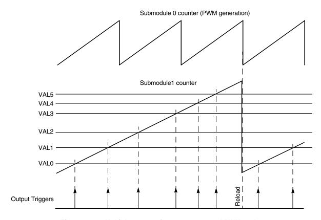
Figure 25-35. Multiple output triggers over several PWM cycles
