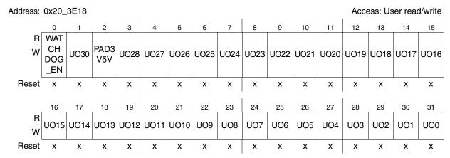
Figure 17-32. Non-Volatile User Options register (NVUSRO)
