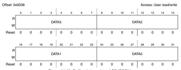
Figure 21-20. Buffer data register LSB (BDRL)
