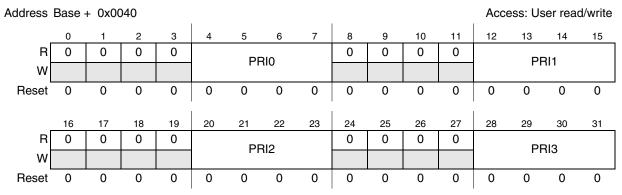
Figure 9-8. INTC Priority Select Register 0-3 (INTC\_PSR[0:3])
