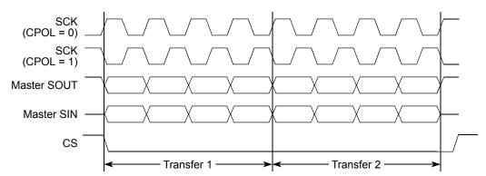
Figure 20-24. Continuous SCK timing diagram (CONT = 1)
