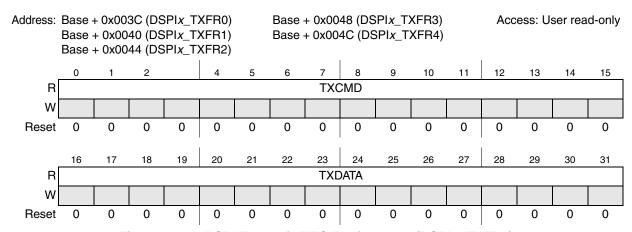
Figure 20-10. DSPI Transmit FIFO Register 0–4 (DSPIx\_TXFRn)
