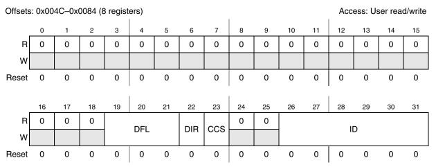
Figure 21-25. Identifier filter control register (IFCR2n)
