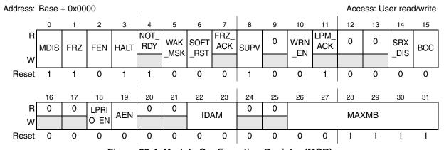
Figure 22-4. Module Configuration Register (MCR)
