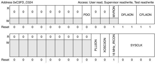
Figure 7-10. TEST Mode Configuration Register (ME\_TEST\_MC)
