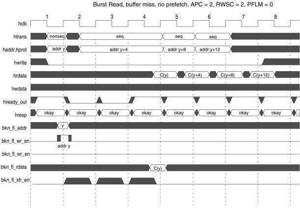
Figure 17-4. 3-cycle access, no prefetch, buffering enabled
