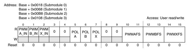
Figure 25-13. Output Control register (OCTRL)
