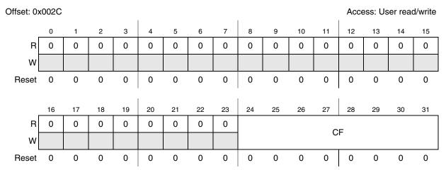
Figure 21-17. LIN checksum field register (LINCFR)
