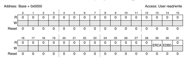
Figure 18-2. eDMA Control Register (EDMA\_CR)
