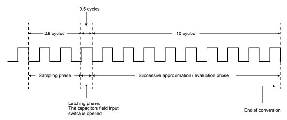
Note: Operating conditions — INPLATCH = 0, INPSAMP = 3, INPCMP = 1 and Fadc clk = 20 MHz
