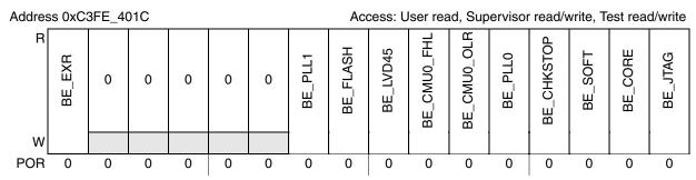
Figure 8-8. Functional Bidirectional Reset Enable Register (RGM\_FBRE)
