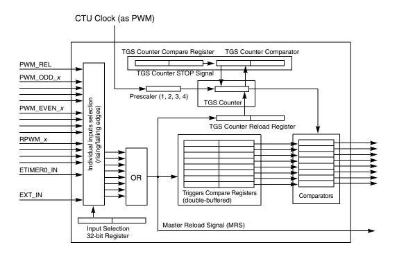
Figure 24-2. TGS in triggered mode
