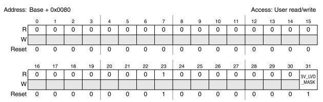
Figure 34-1. Voltage Regulator Control register (VREG\_CTL)
