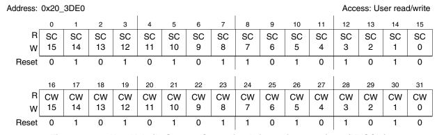
Figure 17-30. Non-Volatile System Censoring Information 0 register (NVSCI0)
