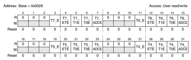
Figure 24-17. Trigger handler control register 2 (THCR2)
