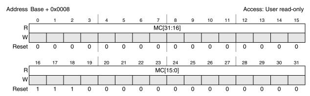
Figure 15-5. IPS Module Configuration (IMC) register
