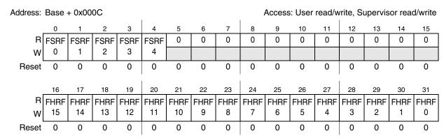
Figure 28-6. Fake Fault Generation Register (FCU\_FFGR)
