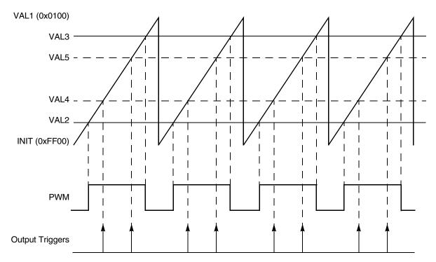
Figure 25-34. Multiple output trigger generation in hardware
