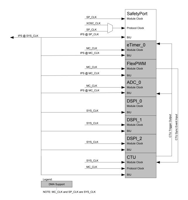
Figure 4-2. MPC5602P system clock distribution Part A
