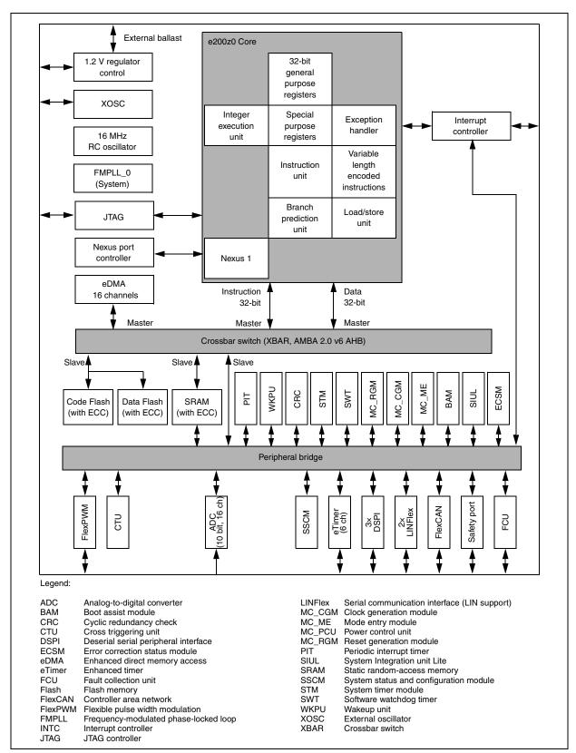
Figure 1-3. MPC5602P block diagram
