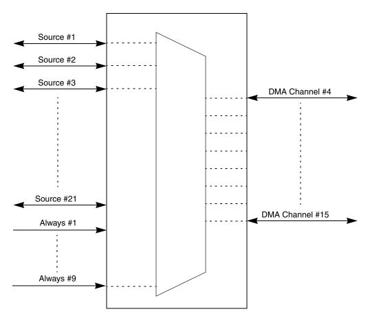
Figure 19-6. DMA mux channel 4-15 block diagram
