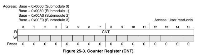
This read-only register displays the state of the signed 16-bit submodule counter. This register is not byte accessible
