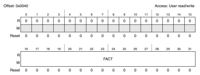
Figure 21-22. Identifier filter enable register (IFER)
