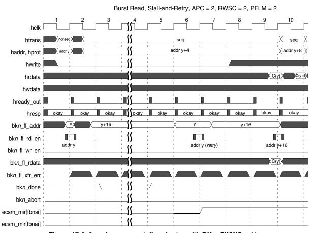
Figure 17-6. 3-cycle access, stall-and-retry with  $BKn_RWWC = 11x$
