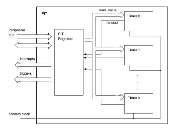
Figure 30-1. PIT block diagram
