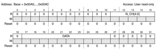
Figure 24-25. FIFO signed Left aligned data x (x = 0,...,3) (FLx)
