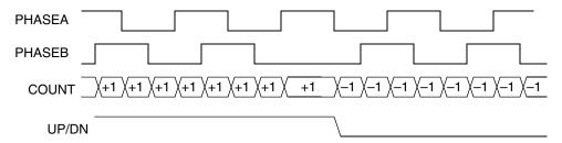
Figure 26-24. Quadrature incremental position encoder
