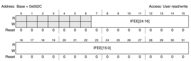
Figure 11-8. Interrupt Falling-Edge Event Enable Register (IFEER)
