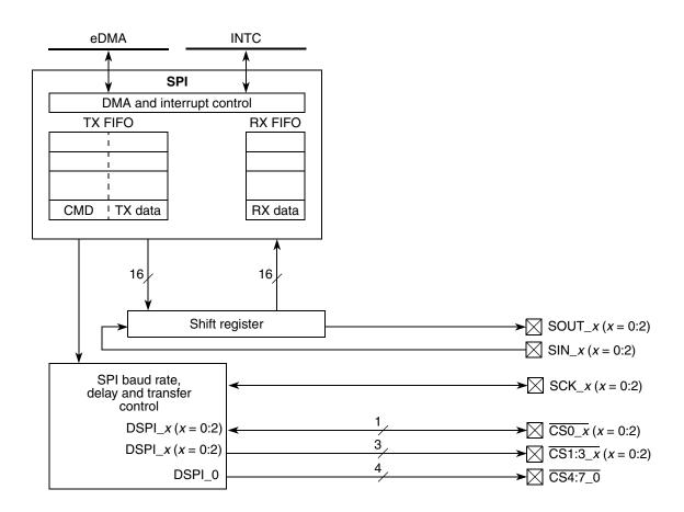
Figure 20-1. DSPI block diagram
