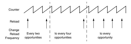
Figure 25-55. Half cycle reload frequency change
