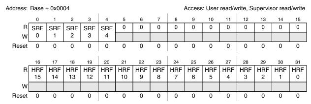
Figure 28-4. Fault Flag Register (FCU\_FFR)
