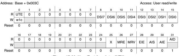
Figure 17-20. User Test 0 register (UT0)
