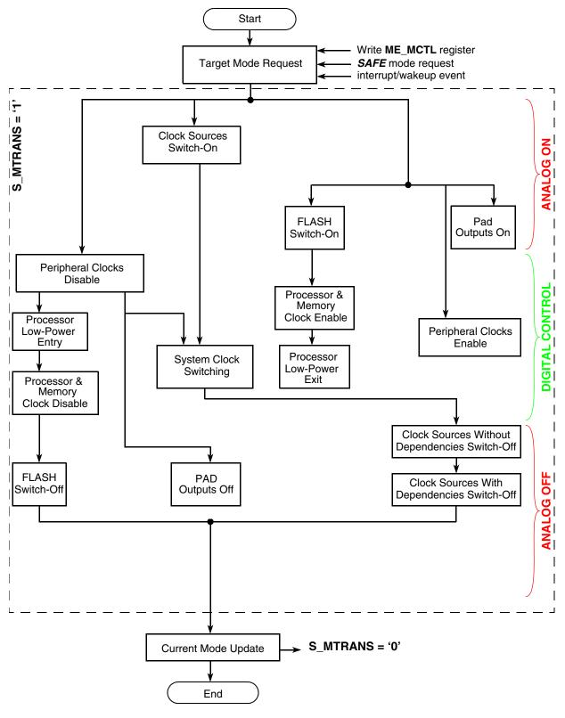
Figure 7-23. MC\_ME Transition Diagram
