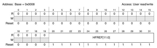
Figure 4-14. High Frequency Reference register FMPLL\_0 (CMU\_0\_HFREFR\_A)
