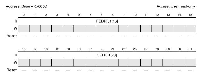
Figure 15-15. Flash ECC Data register (FEDR)
