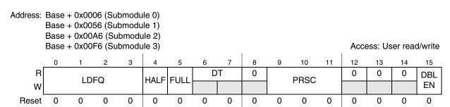
Figure 25-6. Control 1 Register (CTRL1)
