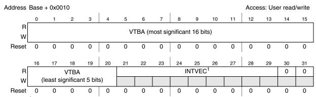
When the VTES bit in INTC\_MCR is asserted, INTVEC is shifted to the left one bit. Bit 29 is read as a '0'. VTBA is narrowed to 20 bits in width.
