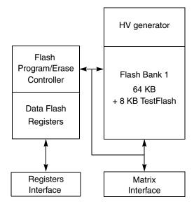
Figure 17-8. Data Flash module structure
