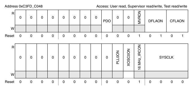
Figure 7-15. STOP0 Mode Configuration Register (ME\_STOP0\_MC)
