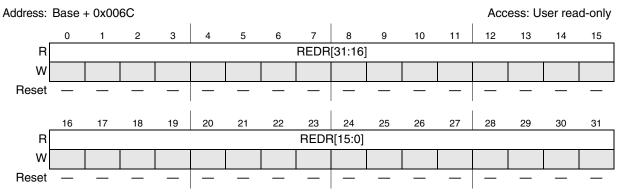
Figure 15-20. Platform RAM ECC Data register (PREDR)
