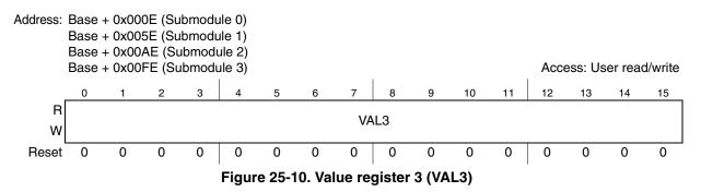
The 16-bit signed value in this register defines the count value to set PWMA low (Figure 25-2). This register is not byte accessible.
