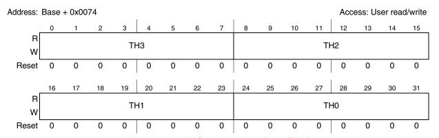
Figure 24-22. FIFO threshold register (FTH)
