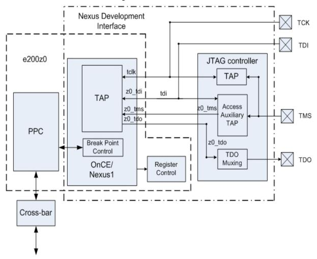
Figure 36-1. NDI functional block diagram
