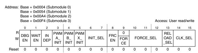
Figure 25-5. Control 2 Register (CTRL2)
