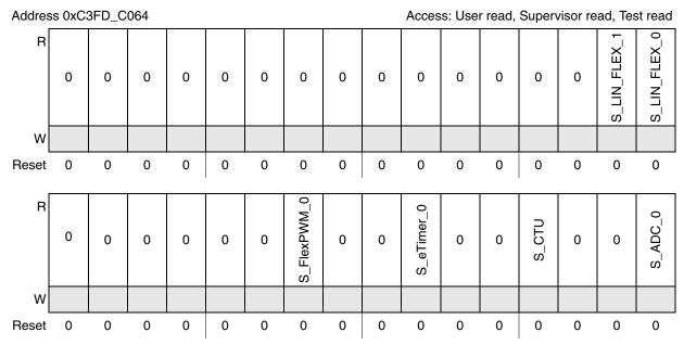
Figure 7-17. Peripheral Status Register 1 (ME\_PS1)
