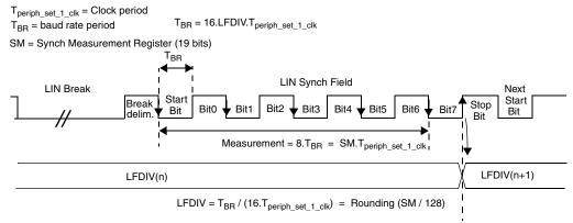
Figure 21-31. LIN synch field measurement
