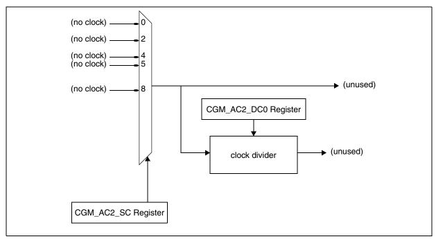
Figure 5-15. MC\_CGM Auxiliary Clock 2 Generation Overview
