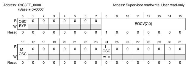
Figure 4-5. Crystal Oscillator Control register (OSC\_CTL)
