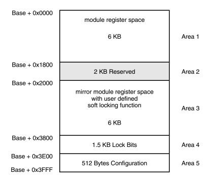
Figure 27-2. Register protection memory diagram
