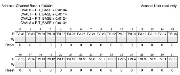
Figure 30-4. Current Timer Value register n (CVALn)
