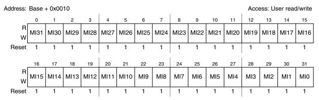
Figure 22-7. Rx Global Mask register (RXGMASK)
