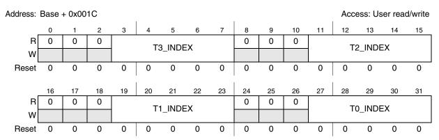
Figure 24-14. Commands list control register 1 (CLCR1)
