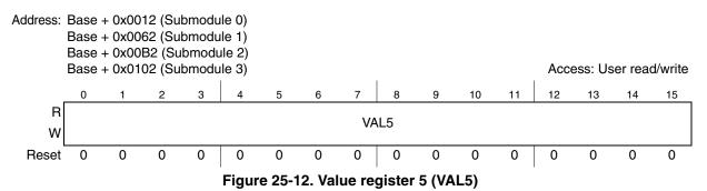
The 16-bit signed value in this register defines the count value to set PWMB low (Figure 25-2). This register is not byte accessible.
