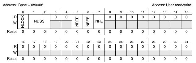
Figure 29-2. NMI Configuration Register (NCR)
