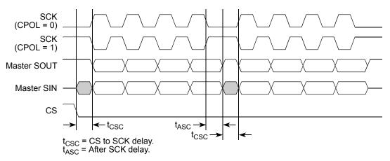
Figure 20-21. Example of continuous transfer (CPHA = 1, CONT = 1)
