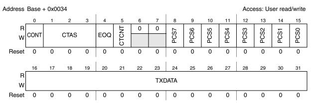
Figure 20-8. DSPI PUSH TX FIFO Register (DSPIx\_PUSHR)
