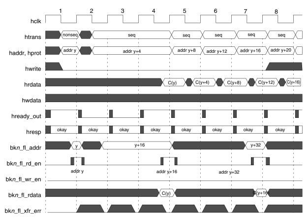
Figure 17-5. 3-cycle access, prefetch and buffering enabled
