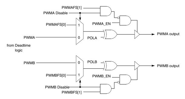
Figure 25-49. Output logic section
