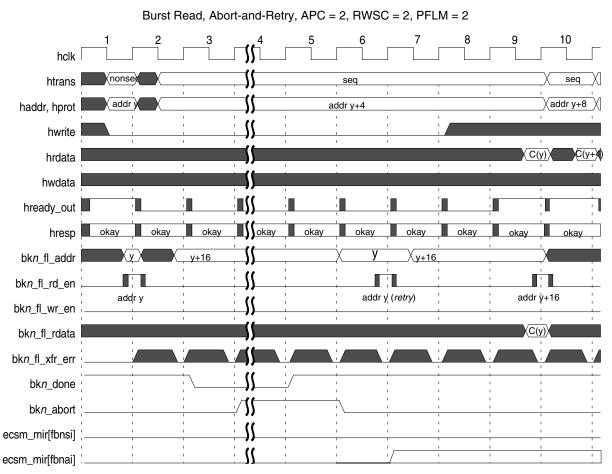
Figure 17-7. 3-cycle access, terminate-and-retry with  $BKn_RWWC = 10x$
