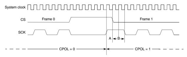
Figure 20-22. Polarity switching between frames
