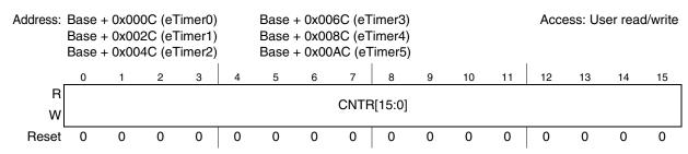
Figure 26-9. Counter register (CNTR)
