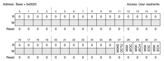
Figure 23-10. Interrupt Mask Register (IMR)
