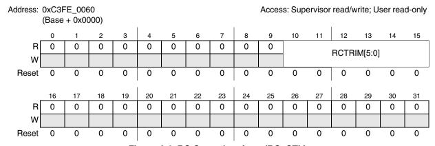
Figure 4-4. RC Control register (RC\_CTL)
