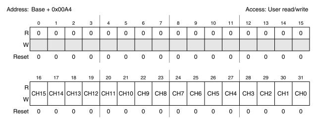
Figure 23-19. Normal Conversion Mask Register 0 (NCMR0)
