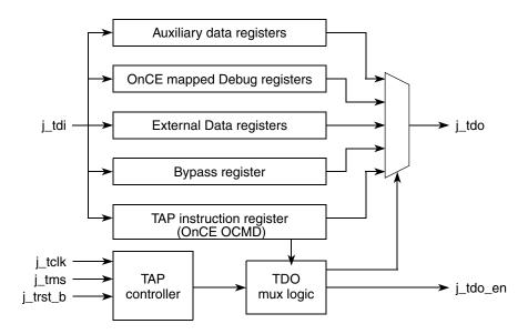
Figure 36-10. OnCE TAP Controller and Registers
