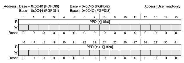
Figure 11-15. Parallel GPIO Pad Data In register 0-3 (PGPDI[0:3])
