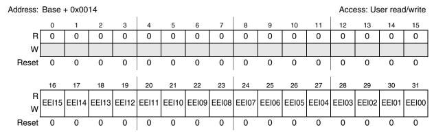
Figure 18-5. eDMA Enable Error Interrupt Low Register (EDMA\_EEIRL)
