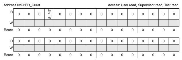
Figure 7-18. Peripheral Status Register 2 (ME\_PS2)
