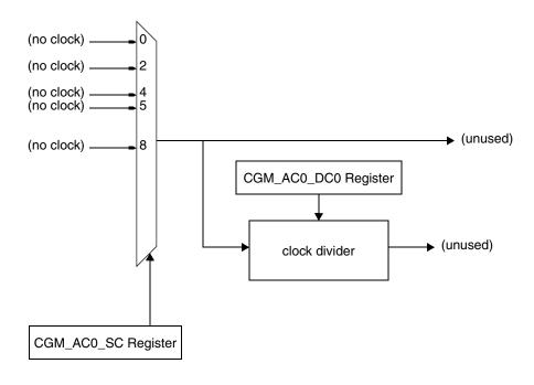
Figure 5-13. MC\_CGM Auxiliary Clock 0 Generation Overview
