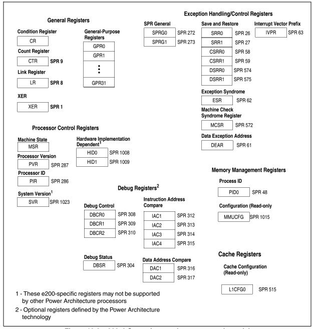
Figure 12-3. e200z0 Supervisor mode programmer's model
