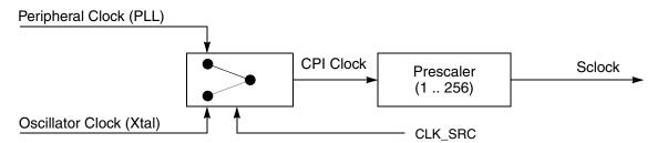
Figure 22-15. CAN engine clocking scheme
