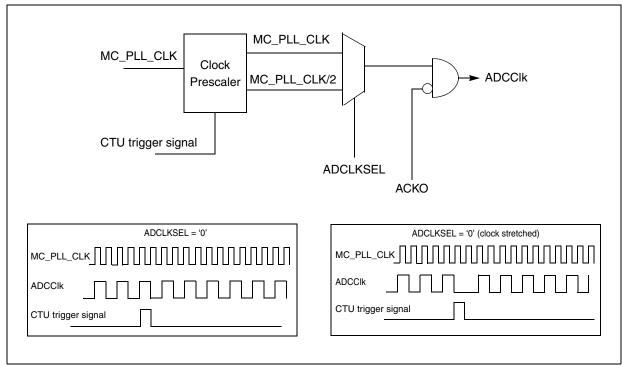
Figure 23-4. Prescaler simplified block diagram
