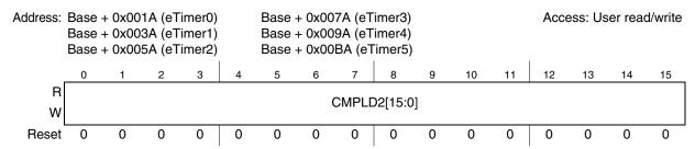
Figure 26-16. Comparator Load 2 (CMPLD2)
