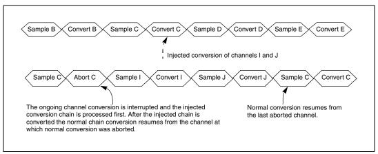
Figure 23-3. Injected sample/conversion sequence
