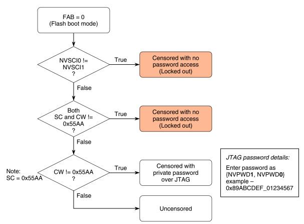
Figure 33-15. Censorship control in flash memory boot mode
