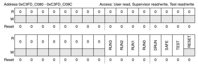
Figure 7-19. Run Peripheral Configuration Registers (ME\_RUN\_PC0...7)
