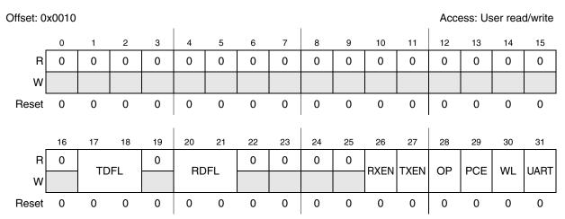
Figure 21-10. UART mode control register (UARTCR)
