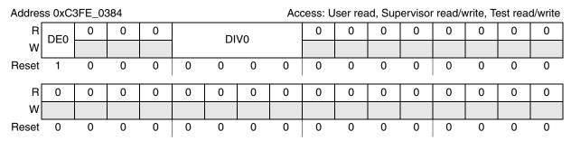
Figure 5-7. Auxiliary Clock 0 Divider Configuration Register (CGM\_AC0\_DC0)
