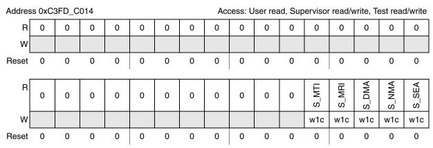
Figure 7-7. Invalid Mode Transition Status Register (ME\_IMTS)
