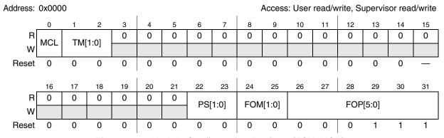
Figure 28-3. Module Configuration Register (FCU\_MCR)
