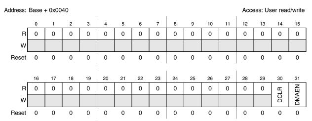
Figure 23-14. DMA Enable (DMAE) register
