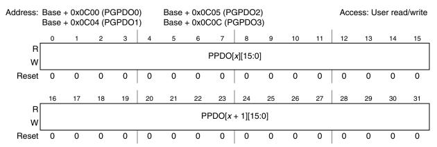
Figure 11-14. Parallel GPIO Pad Data Out register 0-3(PGPDO[0:3])
