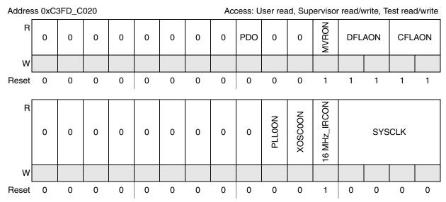
Figure 7-9. RESET Mode Configuration Register (ME\_RESET\_MC)
