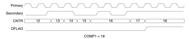
Figure 26-25. Triggered Count mode (length = 1)
