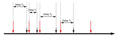
Figure 24-5. Example timing for TGS in sequential mode
