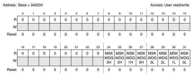
Figure 23-13. Watchdog Threshold Interrupt Mask Register (WTIMR)
