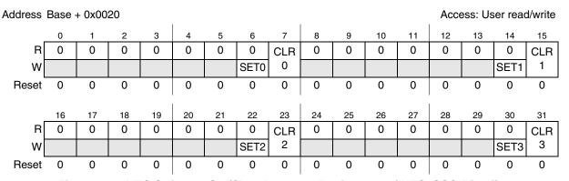
Figure 9-6. INTC Software Set/Clear Interrupt Register 0-3 (INTC\_SSCIR[0:3])
