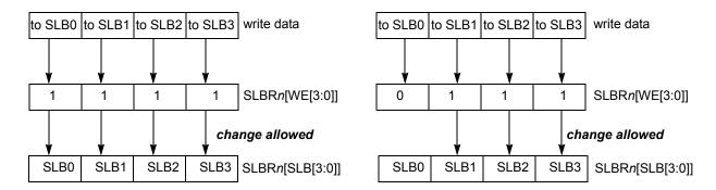
Figure 27-5. Change lock settings directly via area #4
