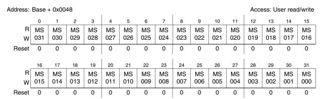
Figure 17-23. User Multiple Input Signature Register 0 (UMISR0)
