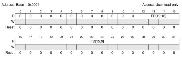
Figure 4-13. Frequency Display Register (CMU\_0\_FDR)
