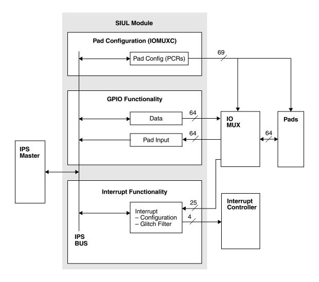
Figure 11-1. System Integration Unit Lite block diagram
