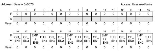
Figure 24-21. FIFO control register (FCR)
