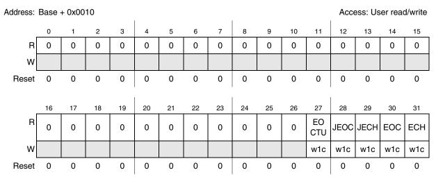
Figure 23-9. Interrupt Status Register (ISR)
