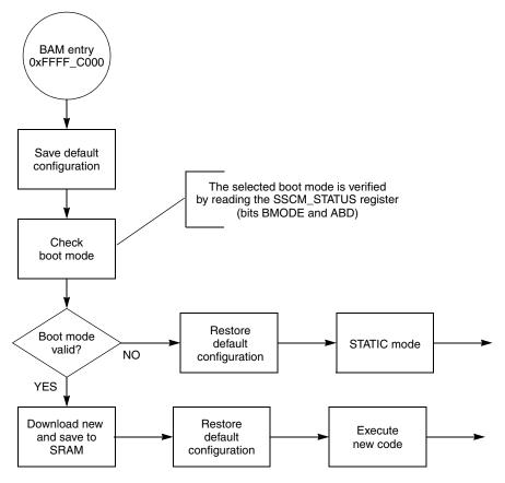
Figure 33-4. BAM logic flow
