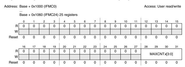
Figure 11-17. Interrupt Filter Maximum Counter registers 0-24 (IFMC[0:24])
