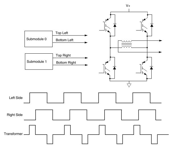
Figure 25-32. Phase-shifted PWMs applied to a transformer primary
