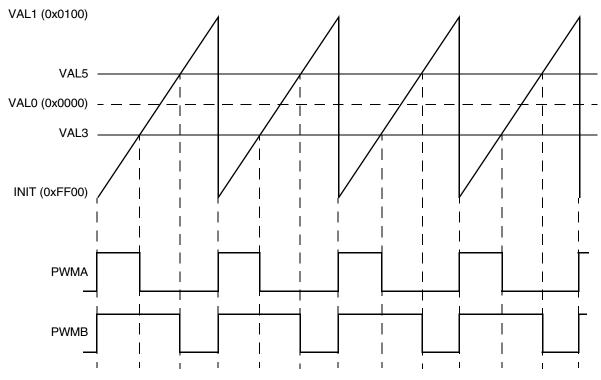
Figure 25-30. Edge-aligned example (INIT = VAL2 = VAL4)
