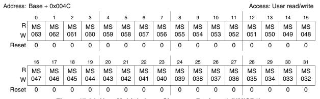
Figure 17-24. User Multiple Input Signature Register 1 (UMISR1)
