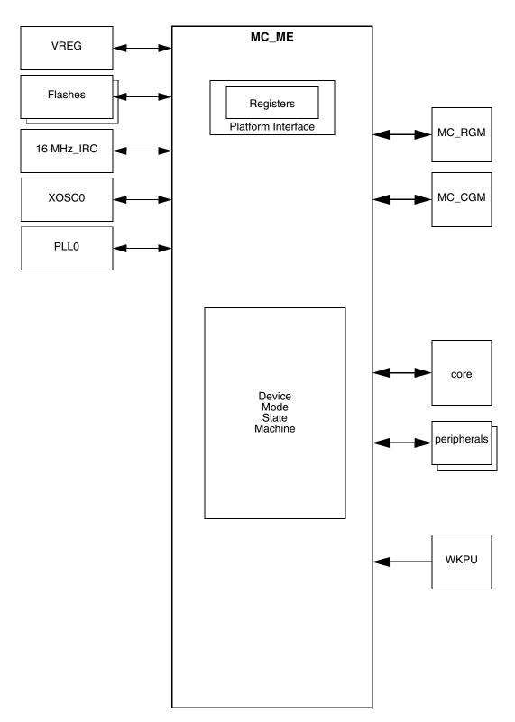
Figure 7-1. MC\_ME Block Diagram
