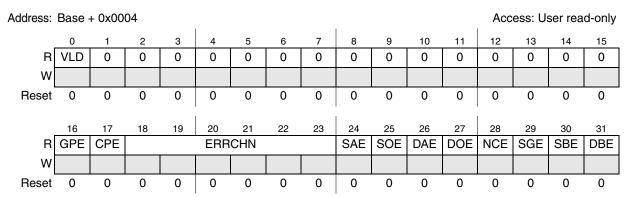
Figure 18-3. eDMA Error Status Register (EDMA\_ESR)
