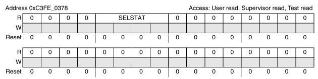
Figure 5-4. System Clock Select Status Register (CGM\_SC\_SS)
