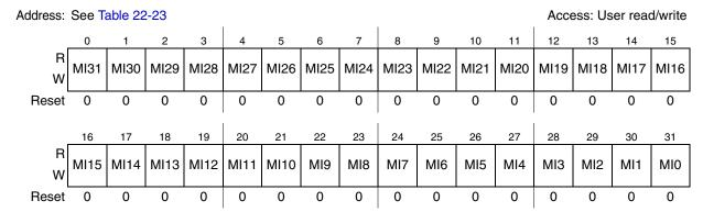
Figure 22-14. Rx Individual Mask Registers (RXIMR0-RXIMR31)
