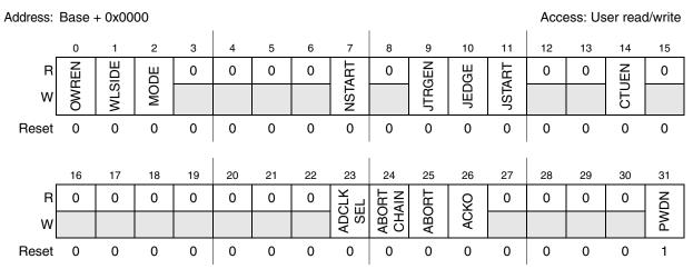
Figure 23-7. Main Configuration Register (MCR)
