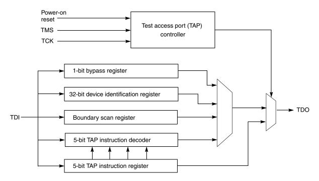
Figure 35-1. JTAG controller block diagram
