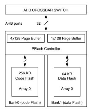
Figure 17-1. MPC5602P Flash memory architecture
