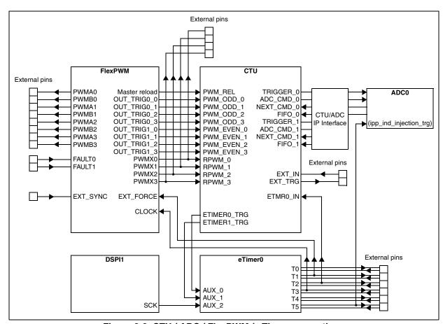
Figure 3-3. CTU / ADC / FlexPWM / eTimer connections
