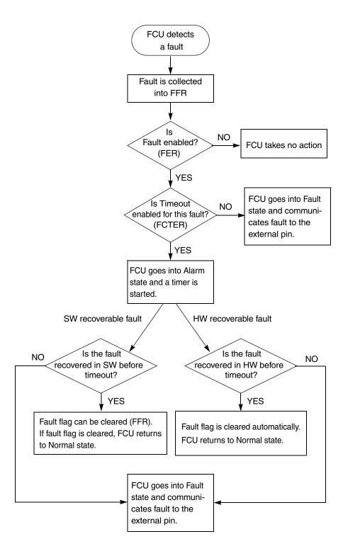
Figure 28-2. FCU fault handling
