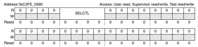
Figure 5-10. Auxiliary Clock 2 Select Control Register (CGM\_AC2\_SC)
