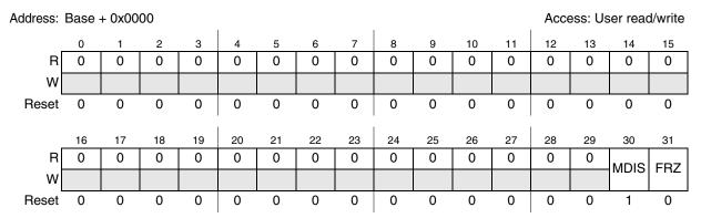
Figure 30-2. PIT Module Control Register (PITMCR)
