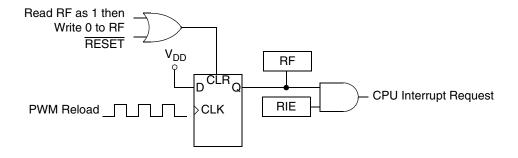
Figure 25-57. PWMF reload interrupt request
