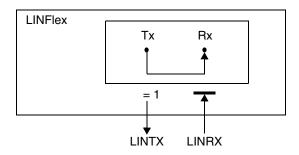
Figure 21-5. LINFlex in self test mode
