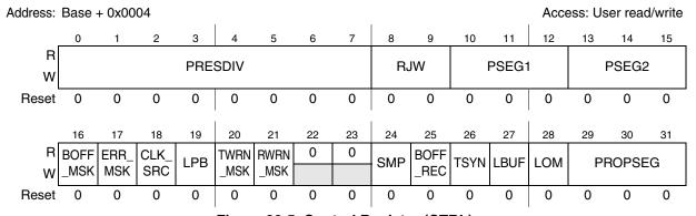
Figure 22-5. Control Register (CTRL)
