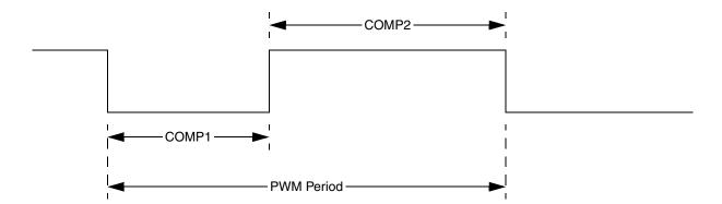
Figure 26-28. Variable PWM waveform
