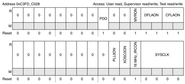
Figure 7-11. SAFE Mode Configuration Register (ME\_SAFE\_MC)
