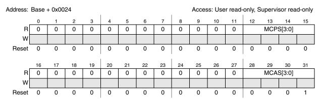
Figure 28-12. MC State Register (FCU\_MCSR)
