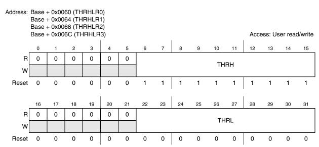
Figure 23-17. Threshold Register (THRHLR[0:3])
