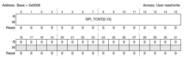
Figure 20-4. DSPI Transfer Count Register (DSPIx\_TCR)
