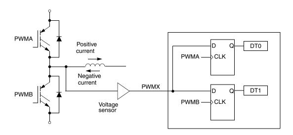
Figure 25-47. Current-status sense scheme for deadtime correction
