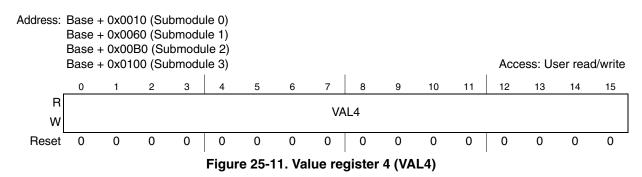
The 16-bit signed value in this register defines the count value to set PWMB high (Figure 25-2). This register is not byte accessible.
