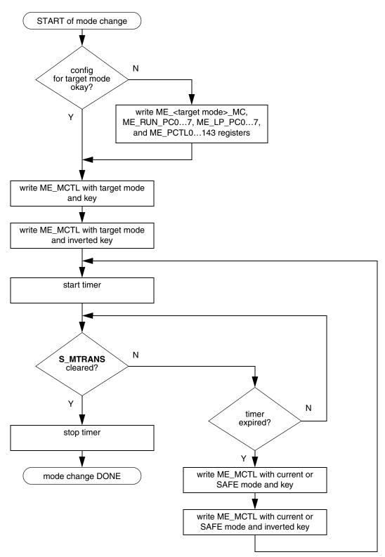
Figure 7-24. MC\_ME Application Example Flow Diagram
