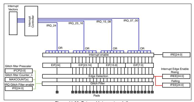
Figure 11-20. External interrupt pad diagram
