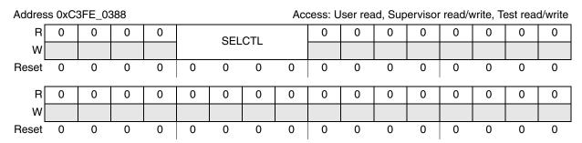
Figure 5-8. Auxiliary Clock 1 Select Control Register (CGM\_AC1\_SC)
