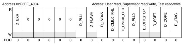
Figure 8-4. Functional Event Reset Disable Register (RGM\_FERD)
