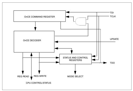
Figure 36-12. e200z0h OnCE Controller and Serial Interface
