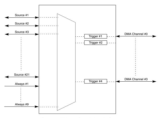
Figure 19-3. DMA mux triggered channels diagram
