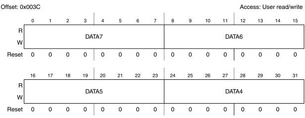
Figure 21-21. Buffer data register MSB (BDRM)
