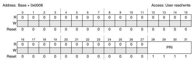
Figure 9-3. INTC Current Priority Register (INTC\_CPR)
