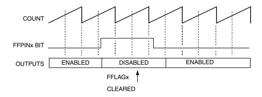
Figure 25-53. Manual fault clearing (FSAFE = 1)
