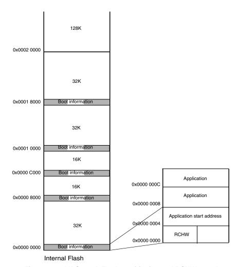
Figure 33-3. MPC5602P Flash partitioning and RCHW search
