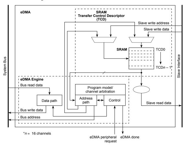
Figure 18-1. eDMA block diagram
