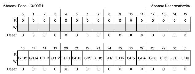
Figure 23-20. Injected Conversion Mask Register 0 (JCMR0)
