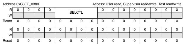
Figure 5-6. Auxiliary Clock 0 Select Control Register (CGM\_AC0\_SC)
