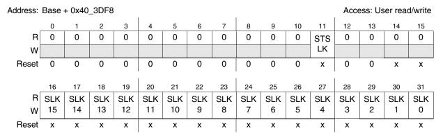
Figure 17-14. Non-Volatile Secondary Low/Mid Address Space Block Locking register (NVSLL)
