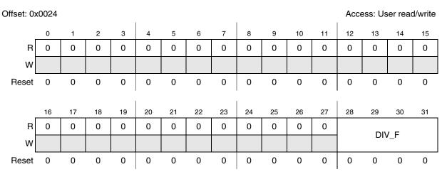
Figure 21-15. LIN fractional baud rate register (LINFBRR)
