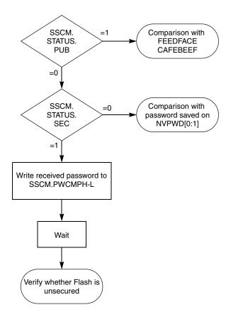
Figure 33-5. Password check flow
