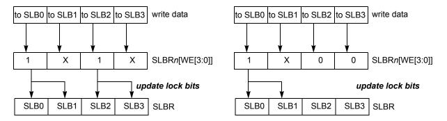
Figure 27-6. Change lock settings for 16-bit protected addresses
