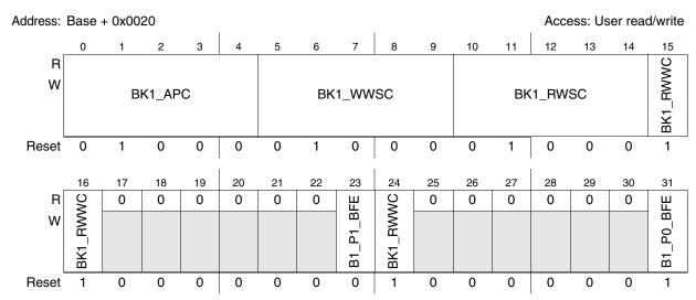
Figure 17-18. Platform Flash Configuration Register 1 (PFCR1)
