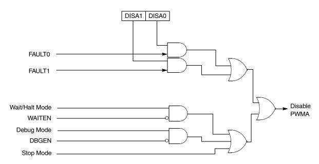
Figure 25-50. Fault decoder for PWMA
