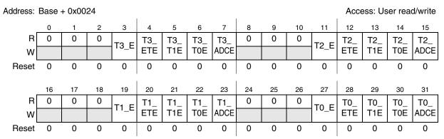
Figure 24-16. Trigger handler control register 1 (THCR1)
