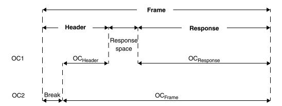
Figure 21-32. Header and response timeout
