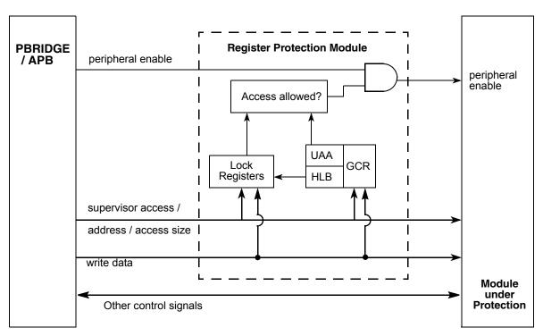
Figure 27-1. Register protection module block diagram
