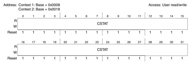
Figure 32-6. CRC Current Status Register (CRC\_CSTAT)
