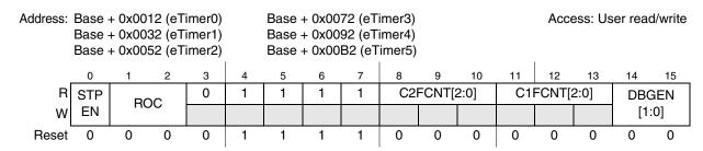
Figure 26-12. Control register 3 (CTRL3)
