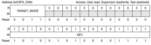
Figure 7-3. Mode Control Register (ME\_MCTL)
