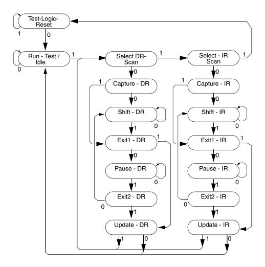
NOTE: The value shown adjacent to each state transition in this figure represents the value of TMS at the time of a rising edge of TCK.
