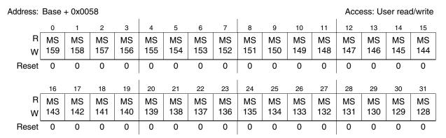
Figure 17-27. User Multiple Input Signature Register 4 (UMISR4)
