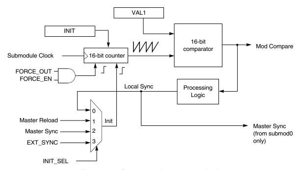
Figure 25-39. Submodule timer synchronization
