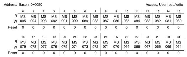
Figure 17-25. User Multiple Input Signature Register 2 (UMISR2)
