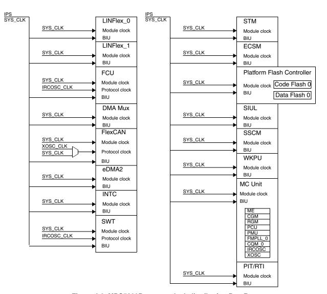
Figure 4-3. MPC5602P system clock distribution Part B
