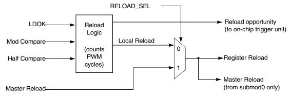
Figure 25-38. Register reload logic
