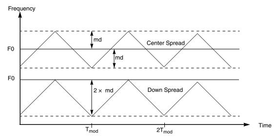
Figure 4-10. Frequency modulation depth spreads
