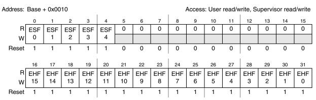
Figure 28-7. Fault Enable Register (FCU\_FER)
