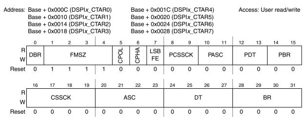
Figure 20-5. DSPI Clock and Transfer Attributes Registers 0-7 (DSPIx\_CTARn)
