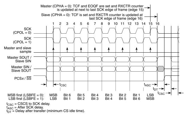
Figure 20-16. DSPI transfer timing diagram (MTFE = 0, CPHA = 0, FMSZ = 8)
