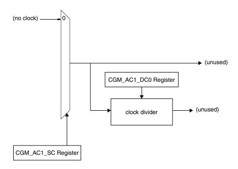
Figure 5-14. MC\_CGM Auxiliary Clock 1 Generation Overview
