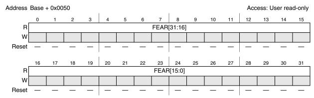
Figure 15-12. Flash ECC Address register (FEAR)
