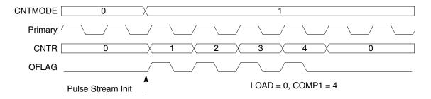
Figure 26-27. Pulse Output mode
