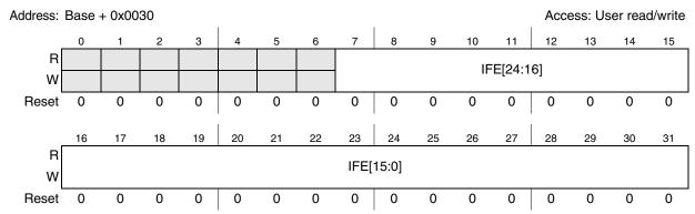
Figure 11-9. Interrupt Filter Enable Register (IFER)
