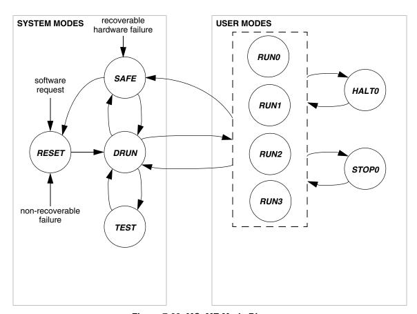
Figure 7-22. MC\_ME Mode Diagram
