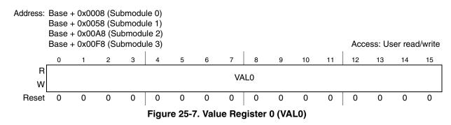
The 16-bit signed value in this buffered, read/write register defines the mid-cycle reload point for the PWM in PWM clock periods. This register is not byte accessible.
