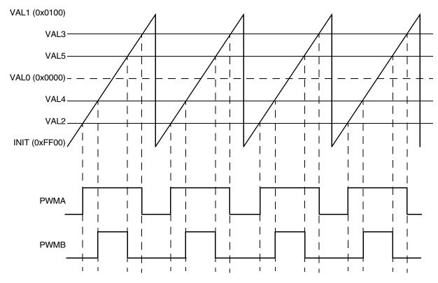
Figure 25-29. Center-aligned example
