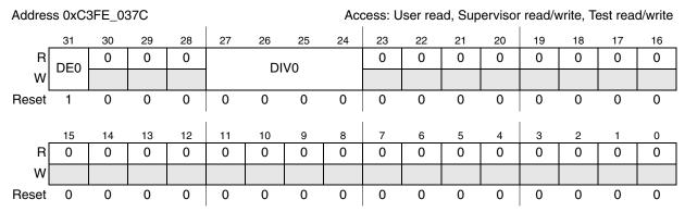
Figure 5-5. System Clock Divider Configuration Register (CGM\_SC\_DC0)
