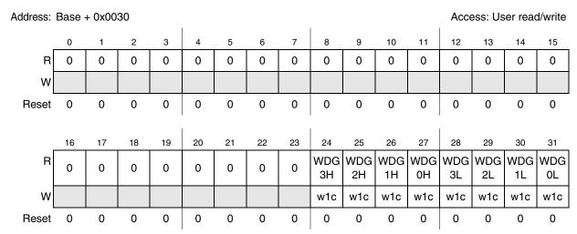
Figure 23-12. Watchdog Threshold Interrupt Status Register (WTISR)
