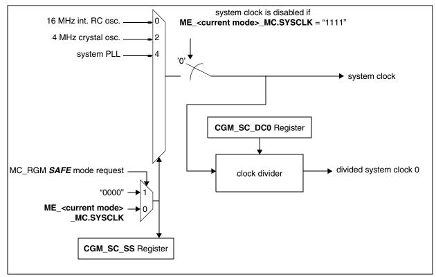
Figure 5-12. MC\_CGM System Clock Generation Overview
