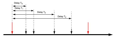
Figure 24-3. Example timing for TGS in triggered mode
