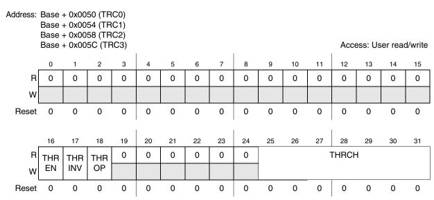
Figure 23-16. Threshold Control Register (TRCx, x = [0..3])
