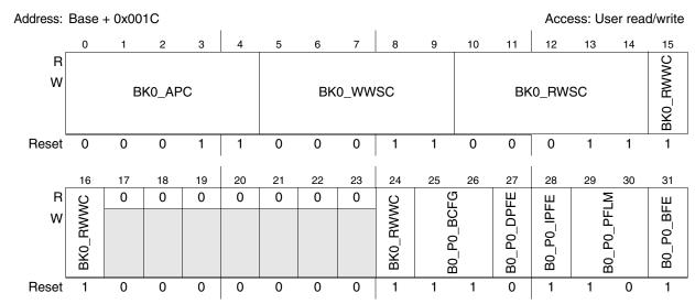
Figure 17-17. Platform Flash Configuration Register 0 (PFCR0)
