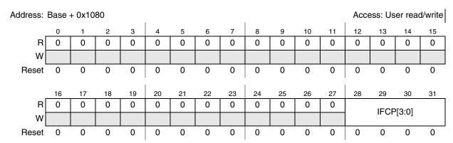
Figure 11-18. Interrupt Filter Clock Prescaler Register (IFCPR)
