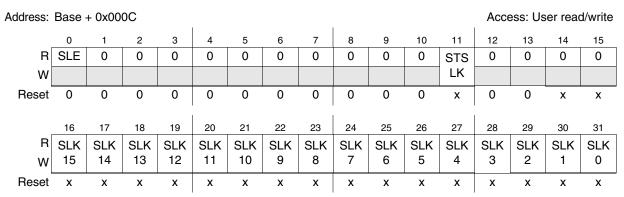
Figure 17-13. Secondary Low/mid address space block Locking reg (SLL)
