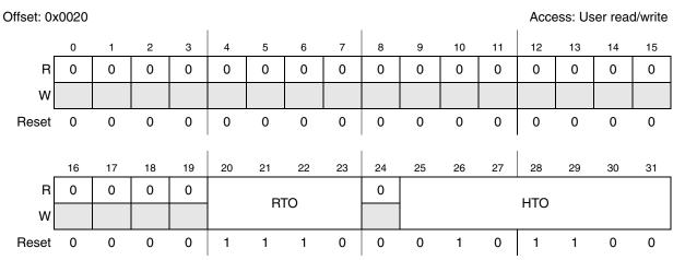
Figure 21-14. LIN timeout control register (LINTOCR)
