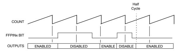
Figure 25-51. Automatic fault clearing
