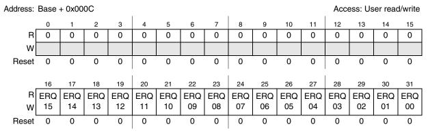
Figure 18-4. eDMA Enable Request Low Register (EDMA ERQRL)
