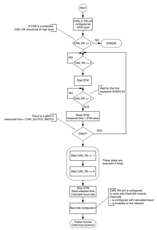
Figure 33-14. BAM rate measurement flow during FlexCAN boot
