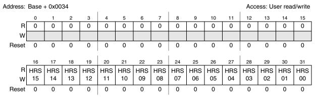
Figure 18-16. EDMA Hardware Request Status Register Low (EDMA\_HRSL)
