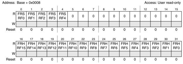
Figure 28-5. Frozen Fault Flag Register (FCU\_FFFR)
