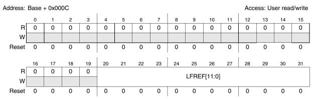
Figure 4-15. Low Frequency Reference Register FMPLL\_0 (CMU\_0\_LFREFR\_A)
