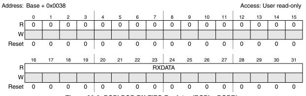
Figure 20-9. DSPI POP RX FIFO Register (DSPIx\_POPR)
