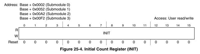
The 16-bit signed value in this register defines the initial count value for the PWM in PWM clock periods. This is the value loaded into the submodule counter when local sync, master sync, or master reload is asserted (based on the value of INIT SEL) or when FORCE is asserted and force init is enabled. For PWM operation, the buffered contents of this register are loaded into the counter at the start of every PWM cycle. This register is not byte accessible.
