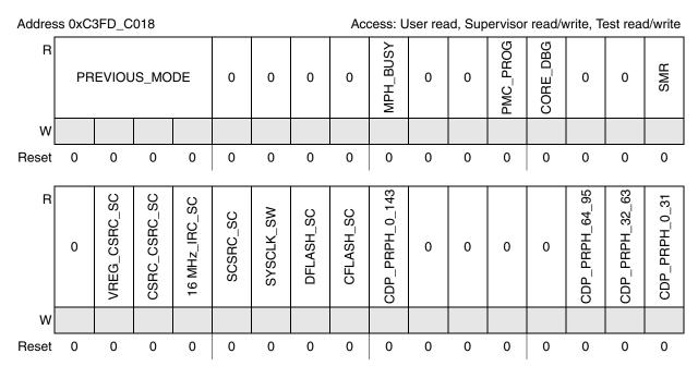
Figure 7-8. Debug Mode Transition Status Register (ME\_DMTS)
