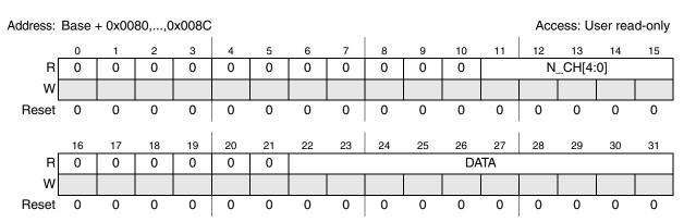
Figure 24-24. FIFO Right aligned data x (x = 0,...,3) (FRx)
