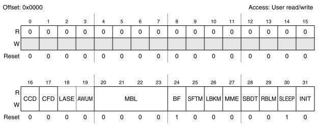
Figure 21-6. LIN control register 1 (LINCR1)
