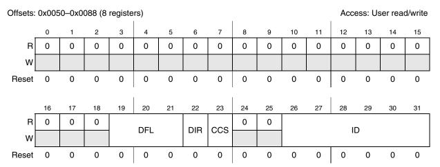
Figure 21-26. Identifier filter control register (IFCR2n + 1)
