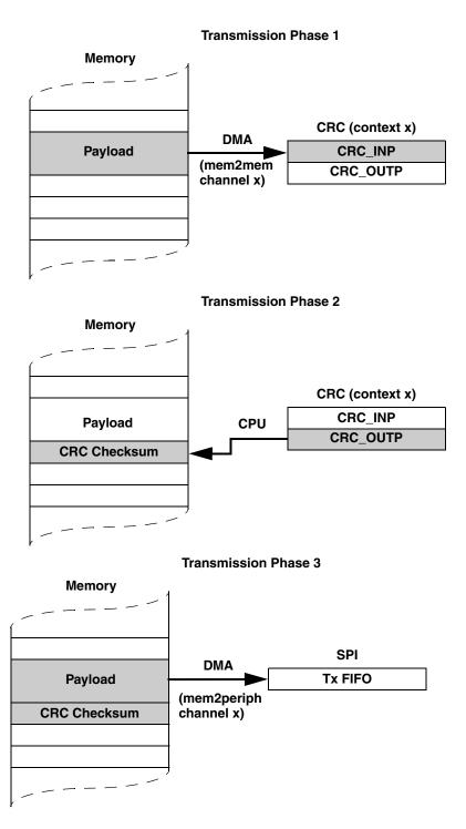
Figure 32-8. DMA-CRC Transmission Sequence
