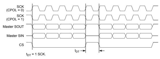
Figure 20-23. Continuous SCK timing diagram (CONT = 0)
