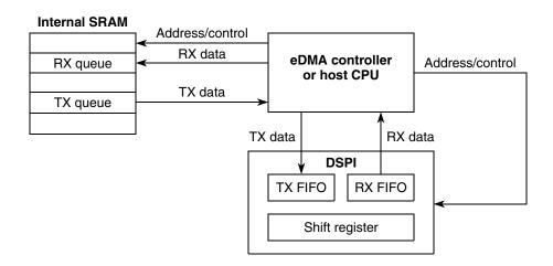
Figure 20-2. DSPI with queues and eDMA
