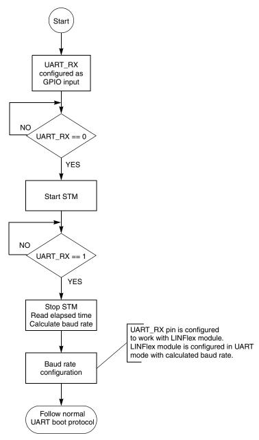
Figure 33-11. BAM rate measurement flow during UART boot
