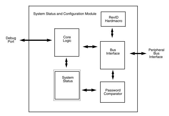
Figure 10-1. SSCM block diagram
