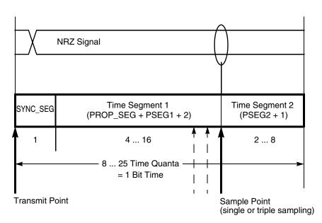
Figure 22-16. Segments within the bit time
