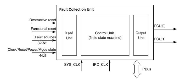
Figure 28-1. Fault Collection Unit (FCU) block diagram
