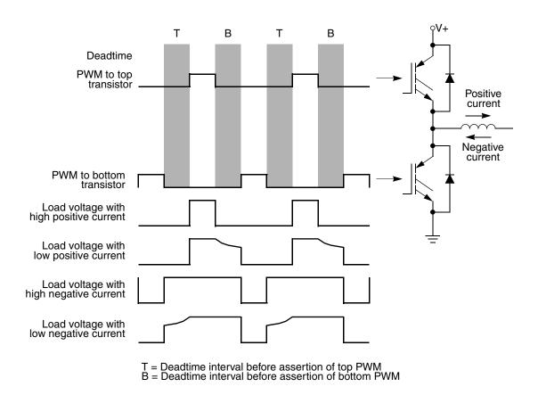
Figure 25-48. Output voltage waveforms
