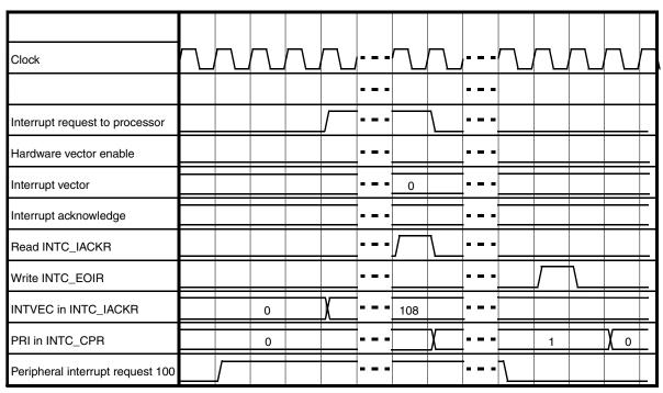
Figure 9-10. Software vector mode handshaking timing diagram
