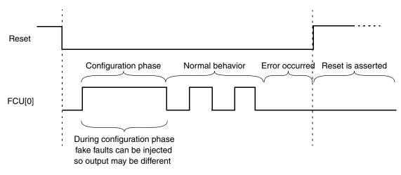
Figure 28-17. Time switching protocol example
