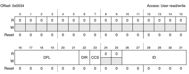
Figure 21-19. Buffer identifier register (BIDR)
