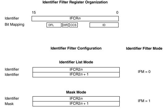
Figure 21-29. Filter configuration—register organization
