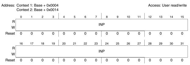
Figure 32-5. CRC Input Register (CRC\_INP)
