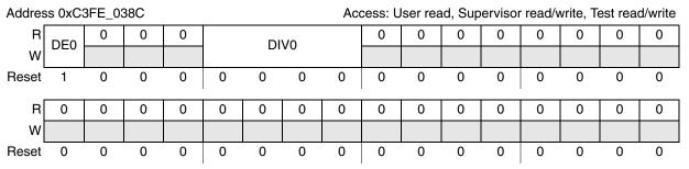
Figure 5-9. Auxiliary Clock 1 Divider Configuration Register (CGM\_AC1\_DC0)
