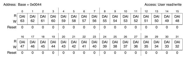
Figure 17-22. User Test 2 register (UT2)
