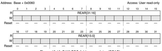
Figure 15-16. RAM ECC Address register (REAR)
