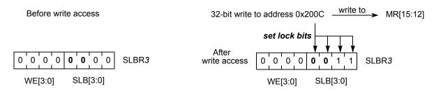
Figure 27-10. Enable locking for protected and unprotected addresses
