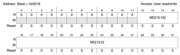
Figure 4-17. Measurement Duration Register (CMU\_0\_MDR)
