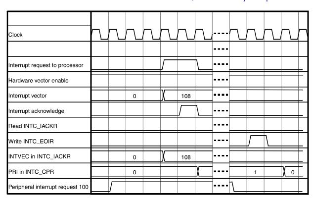
Figure 9-11. Hardware vector mode handshaking timing diagram
