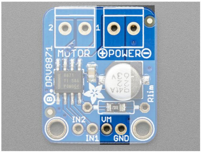
These two sets of pads are connected internally so you can use breadboard or terminal blocks to provide motor power. Use 6.5V-45VDC to power the motor and the chip. This isn't the same as the logic level of the chip, which is up to 5.5 VDC. You do not have to provide a logic level power supply to the chip, how nice is that?
