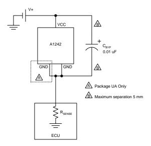
Figure 2. Typical Application Circuit
