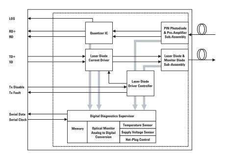
Figure 1. Transceiver Functional Block Diagram
