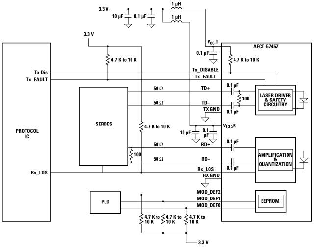
Figure 3. Recommended Application Configuration
