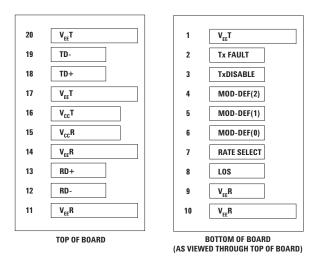
Figure 2. Connection Diagram of Module Printed Circuit Board
