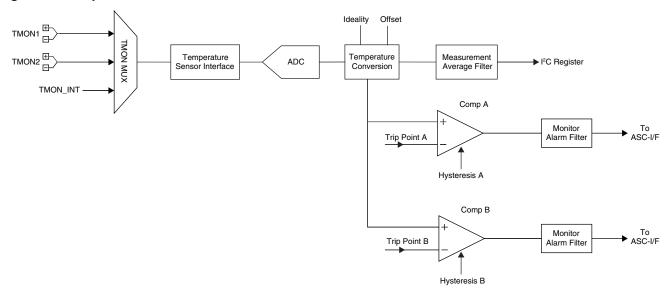
The independently programmable temperature monitor inputs can be used with internal substrate diodes on micro-processors, FPGAs, ASICs, or with low cost external NPN or PNP transistors. The temperature sensor interface block includes programmable support for a variety of sensor configurations as shown in Figure 16. The sensor configuration settings available in the design software are described in Table 13.
