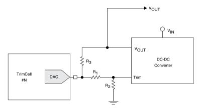
Figure 29 shows an example resistor network between the TrimCell #N in the ASC and the DC-DC converter. The values of these resistors depend on the type of DC-DC converter used and its operating voltage range. The calculation to determine the values of the resistors R1, R2, and R3 is performed automatically in the Platform Designer software.
