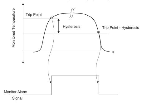
Figure 18. Monitor Alarm Signal Behavior - Undertemperature (UT) Setting
