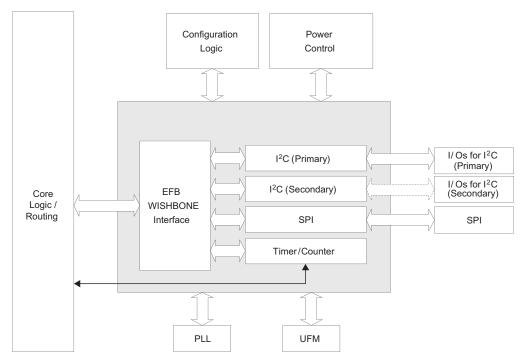
The Platform Manager 2 contains two I<sup>2</sup>C IP cores, the primary and secondary I<sup>2</sup>C IP cores. Each core can be configured either as an I<sup>2</sup>C master or as an I<sup>2</sup>C slave. The main difference between the two IP cores is that the primary core has pre-assigned I/O pin whereas users can assign I/O pins for the secondary core.
