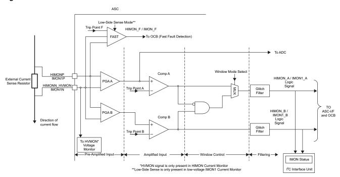
The Current Monitors can be divided into four sections: Pre-Amplified Input, Amplified Input, Window Control, and Filtering. The first section includes the differential input pins IMON1P and IMON1N (low voltage current monitor) or HIMONP and HIMONN\_HVMON (high voltage current monitor). These pins are connected to the PGA circuits as well as the direct differential connection to the Fast Fault Detector.
