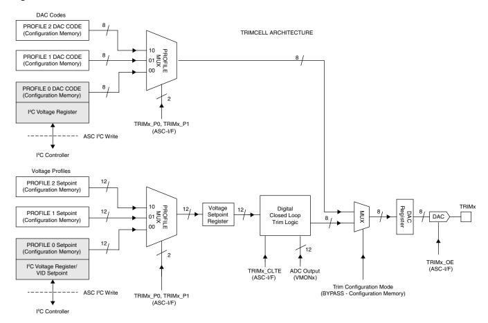
Profile0, Profile1 and Profile2 are 12-bit setpoints, which are written in the EEPROM memory during programming. The active profile for each TrimCell is independently chosen based on ASC-I/F signals TRIMx\_P0 / TRIMx\_P1. This profile is copied to the Voltage Setpoint Register whenever the TRIMx\_P0, TRIMx\_P1 signals change.
