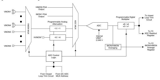
Figure 14 shows the ADC circuit arrangement within the ASC device. The ADC can measure all analog input voltages up to 2.048 V through the multiplexer, ADC MUX. The ADC MUX receives inputs from the High Voltage IMON Programmable Amplifier (PGA), the IMON1 PGA, the High Voltage Monitor (HVMON) at the HIMONN\_HVMON pin, and the VMON MUX. The VMON voltages can be attenuated (divided by three) or unattenuated (divided by
