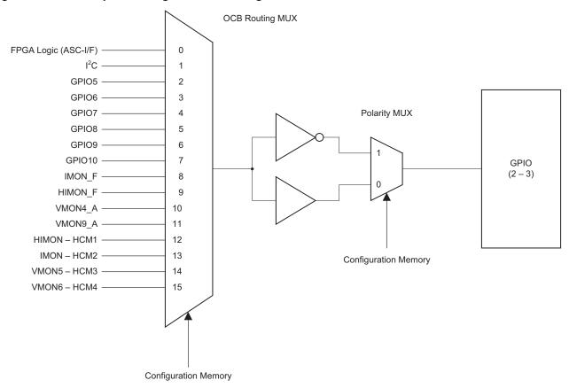
Figure 22 is a generic GPIO routing diagram that applies to GPIO2 & GPIO3 and it provides a bit more detail than the simplified diagram in Figure 20. The MUX on the left is configured by Platform Designer software and selects from either the 12 direct control signals at the top or the four Hysteretic Control Module (HCM) signals at the bottom. The software is also used to select normal or inverted control. The GPIO pin will be on or off based on the Polarity Mux output signal.
