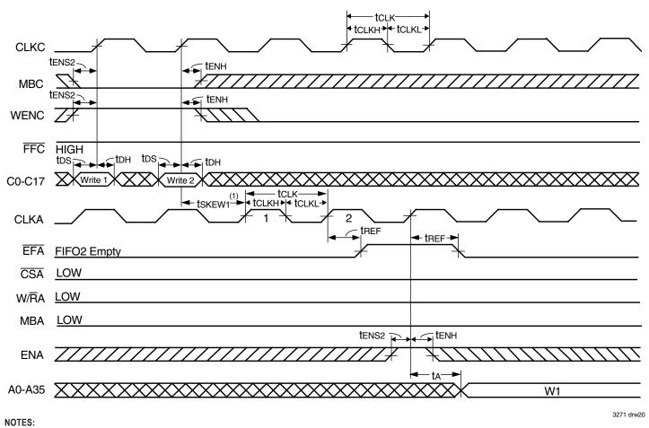
1. tskEw1 is the minimum time between a rising CLKC edge and a rising CLKA edge for EFA to transition HIGH in the next CLKA cycle. If the time between the rising CLKC edge and rising CLKA edge is less than tskEw1, then the transition of EFA HIGH may occur one CLKA cycle later than shown.
