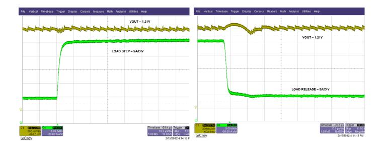
Figure 11. Transient Response – Load Step
