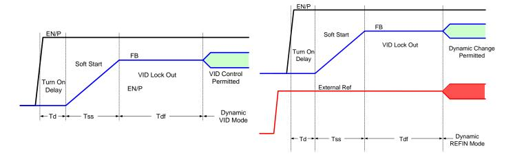
Figure 5. VID Mode Power On Timing
