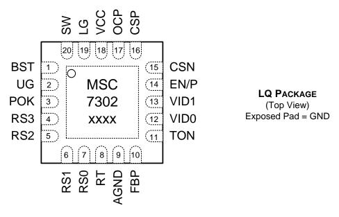
RoHS / Pb-free 100% Matte Tin Finish Figure 3: Pinout
